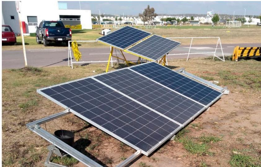
**Figure 13.** Photo of the fixed and tracking systems.
