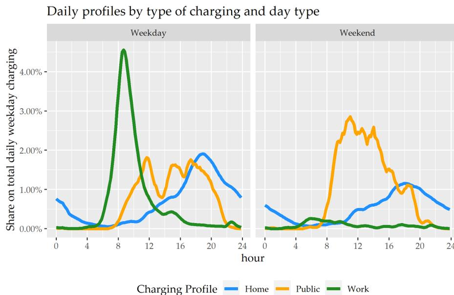
**Figure 1.** Different electric vehicle (EV) charging profiles.
