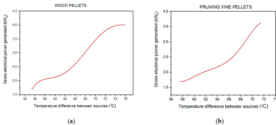
**Figure 3.** Gross electrical power generated in the ORC according to dissipation conditions used: (a) pine pellets and (b) vine pruning pellets.
