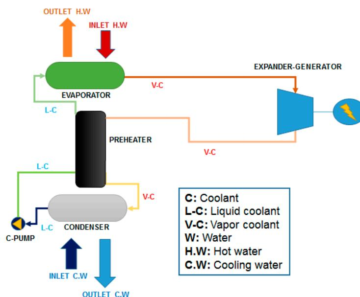
Figure 2. Drawing of the ORC module employed.
