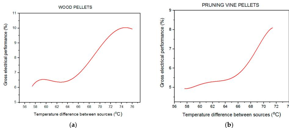
**Figure 4.** Gross electrical performance of the ORC as a function of the dissipation conditions using pine pellets (a) and vine pruning pellets (b).
