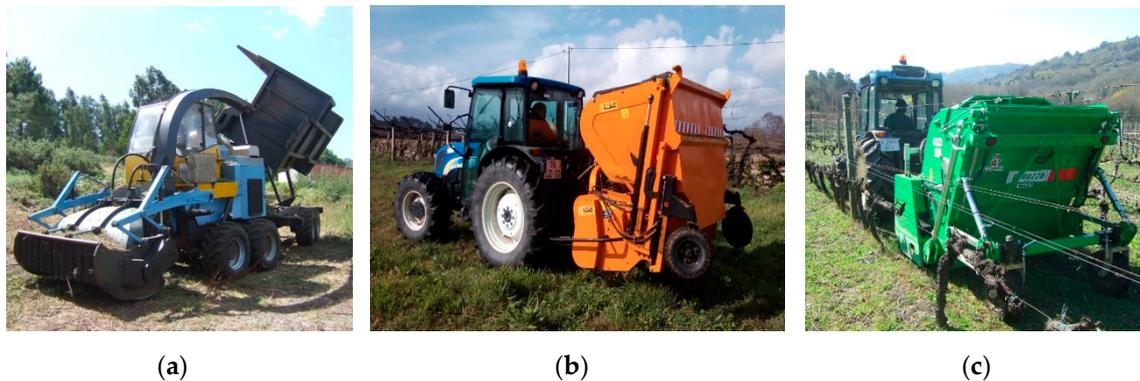
**Figure 1.** Specific machine tested (a) “Retrabio”, (b) Berti Picker and (c) Peruzzo Cobra Collina.
