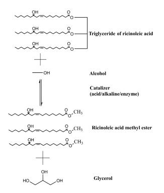
Figure 3. Transesterification reaction during biodiesel production using castor oil as feedstock.
