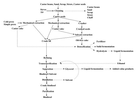
Figure 2. General scheme to produce biodiesel from castor oil (adapted from [40,46]).
