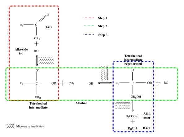
**Figure 1.** Sequence of the transesterification reaction of oil using alkaline catalysis and microwaves (modified from [49]). TAG: Triglyceride, DAG: Diglyceride, R<sub>II</sub>: glyceride, R<sub>I</sub>: carbon chain fatty acid; R: alkyl group of alcohol.
