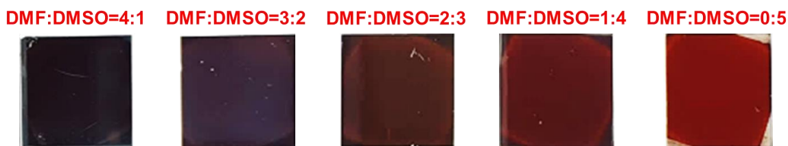
Figure 1. Photographs of lead–tin mixed perovskite films containing different dimethylformamide (DMF)/dimethyl sulfoxide (DMSO) mixed solvent ratios.
