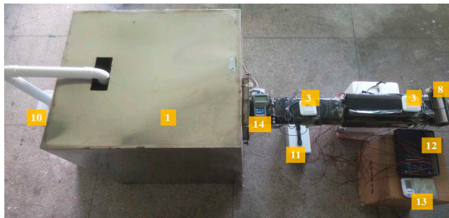
Figure 3. The photo of experimental setup. Notes: 11-DC stabilized power supply 12-Data acquisition instrument 13-Electronic balance 14-Hot wire anemometer.
