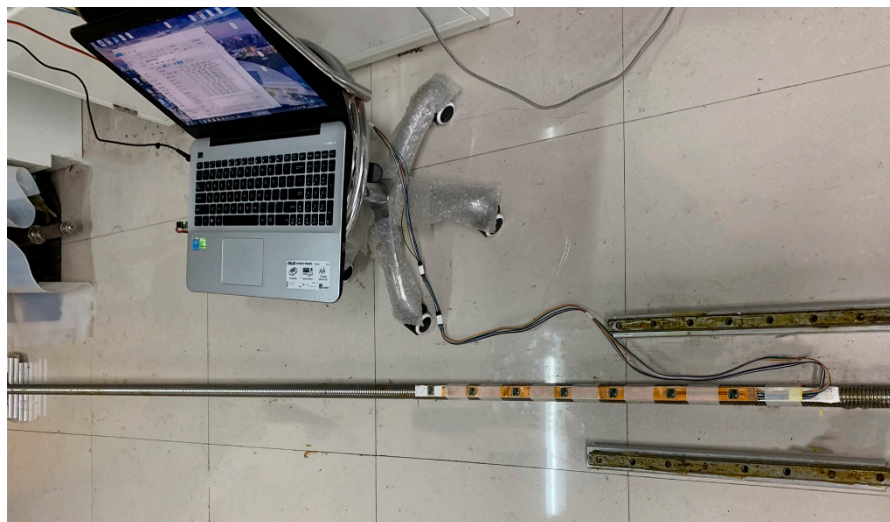
Figure 9. The test of the radial deformation amount of the lead screw.
