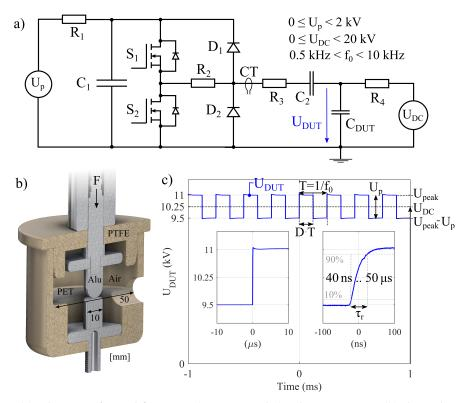
**Figure 1.** (a) Schematic of mixed-frequency (DC + AC pulse) voltage generator; (b) electrode-specimen geometry; (c) exemplary pulse voltage waveform used for time-to-failure testing of polyethylenterephtalat (PET) foil in this study.
