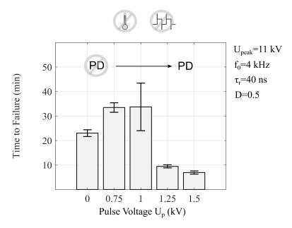
**Figure 4.** Below partial discharge inception voltage (PDIV) ( $U_p < 1 \,\mathrm{kV}$ ), the time to failure increases with increasing pulse voltage  $U_p$  (at fixed peak voltage  $U_{\mathrm{peak}} = 11 \,\mathrm{kV}$ ). Above PDIV ( $U_p > 1 \,\mathrm{kV}$ ), on the other hand, the lifetime decreases with increasing pulse voltage amplitude.
