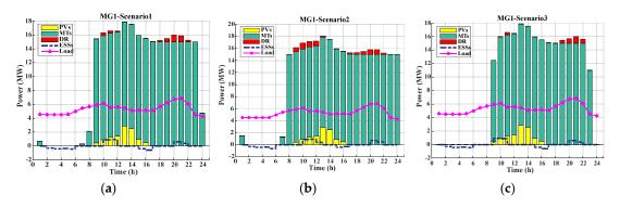
**Figure 6.** Hourly operation scheduling of the MTs, DR programs and ESSs in MG1 for CS1: (a) scenario 1; (b) scenario 2; (c) scenario 3.
