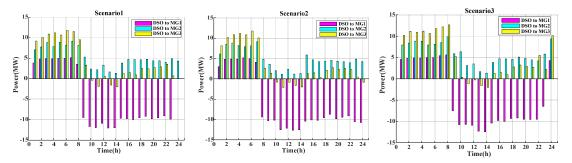
**Figure 10.** Exchanged power between DSO and MGs in different scenarios for CS2: (a) scenario 1; (b) scenario 2; (c) scenario 3.
