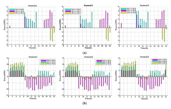
Figure 9. Exchanged power in different scenarios for CS1: (a) among MGs; (b) between DSO and MGs.
