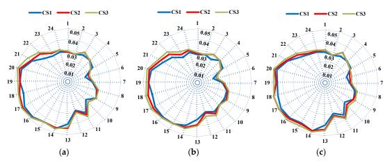
**Figure 14.** The maximum voltage deviation of buses for CS1, CS2 and CS3 in: (a) scenario 1; (b) scenario 2; (c) scenario 3.
