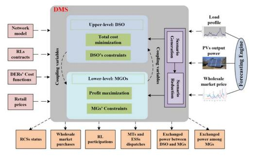
Figure 1. Framework of the proposed bi-level Distribution Management System (DMS).
