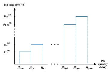
**Figure 2.** A bid-quantity offer package for *i*th node.
