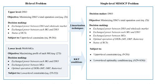
**Figure 3.** Problem statement and its transformation from a bi-level format into a single-level Mixed-Integer Second-Order Cone Programming (MISOCP) problem.
