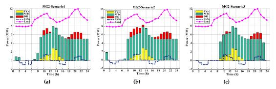
**Figure 7.** Hourly operation scheduling of the MTs, DR programs and ESSs in MG2 for CS1: (a) scenario 1; (b) scenario 2; (c) scenario 3.
