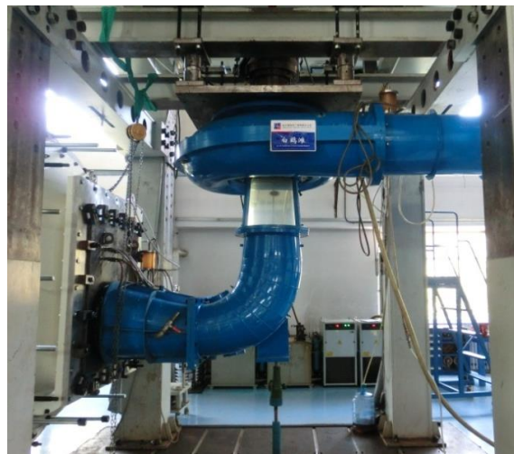
Figure 3. Model Francis turbine of test rig.
