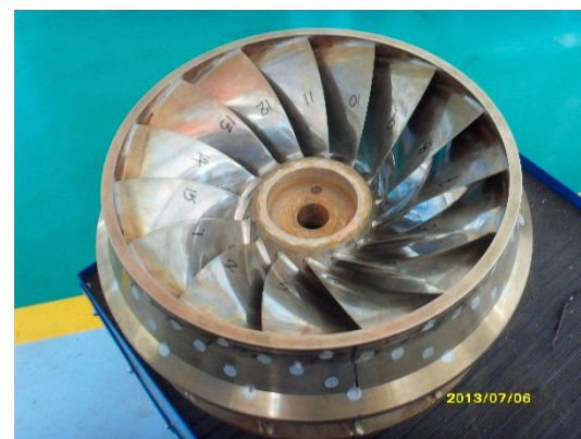
(b) Top view of splitter blades
