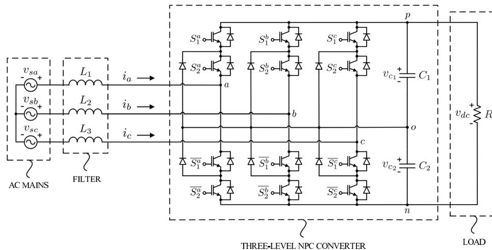
**Figure 1.** Schematic diagram of the three-phase three-level neutral-point-clamped (NPC) rectifier.
