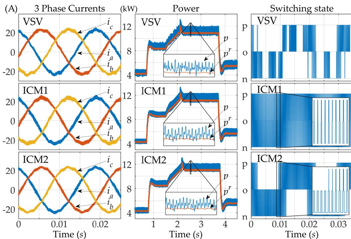
**Figure 6.** Experimental results: (Left) Phase currents at steady state with  $v_{dc} = 800\text{ V}$ ,  $R = 60\ \Omega$  for the mVSVPWM (denoted as VSV in the figure legend), ICM1 and ICM2; (Center) evolution of the instantaneous power ( $p$ ) and its reference ( $p^r$ ) along different operating conditions for the three modulation approaches considered; (Right) switching states at steady state with  $v_{dc} = 800\text{ V}$ ,  $R = 60\ \Omega$  for the three approaches.
