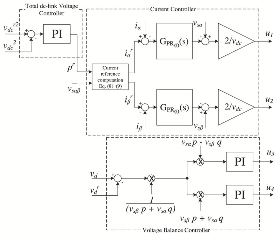
Figure 2. Complete schematic block diagram of the controllers.
