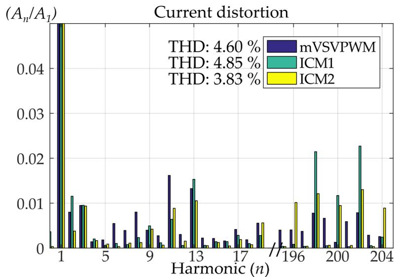
Figure 8. Experimental results: Harmonic spectrum and total harmonic distortion (THD) value of phase *a* current for the three approaches considered: mVSPWM, ICM1 and ICM2.
