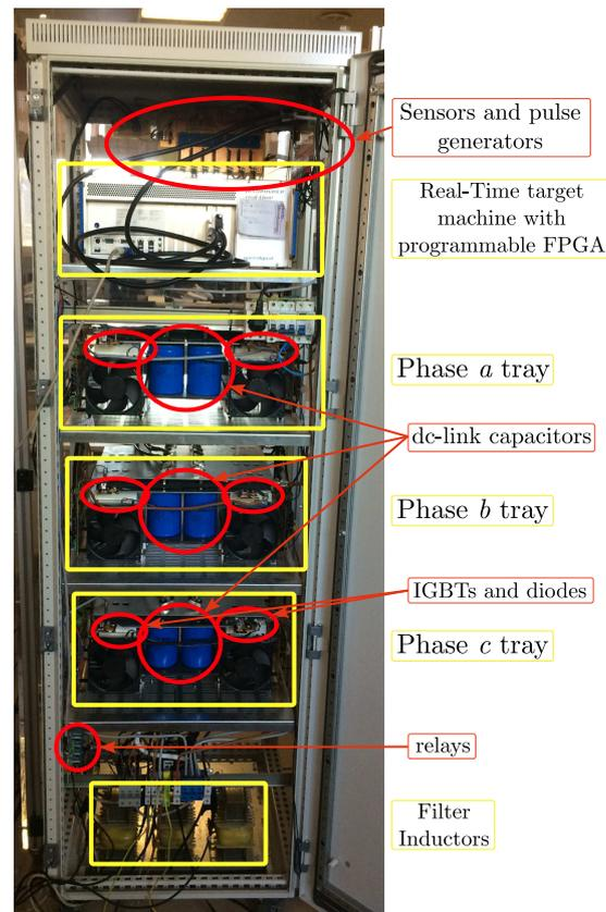
Figure 5. Experimental prototype of the three-level NPC rectifier.
