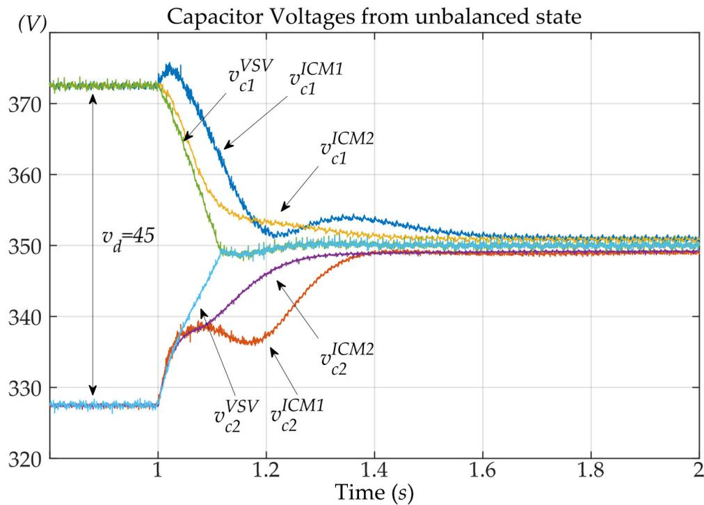
Figure 7. Experimental results: evolution of the capacitor voltages starting from an unbalanced condition, considering mVSPWM (VSV in the figure), ICM1 and ICM2.
