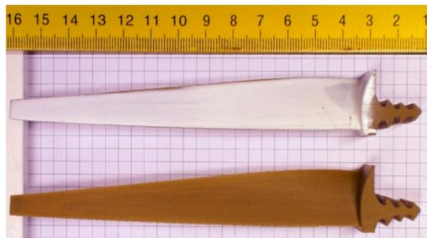
**Figure 6.** A blade before (bottom) and after (top) surface treatment by filling, fine grinding and lacquering; scale in centimeters.
