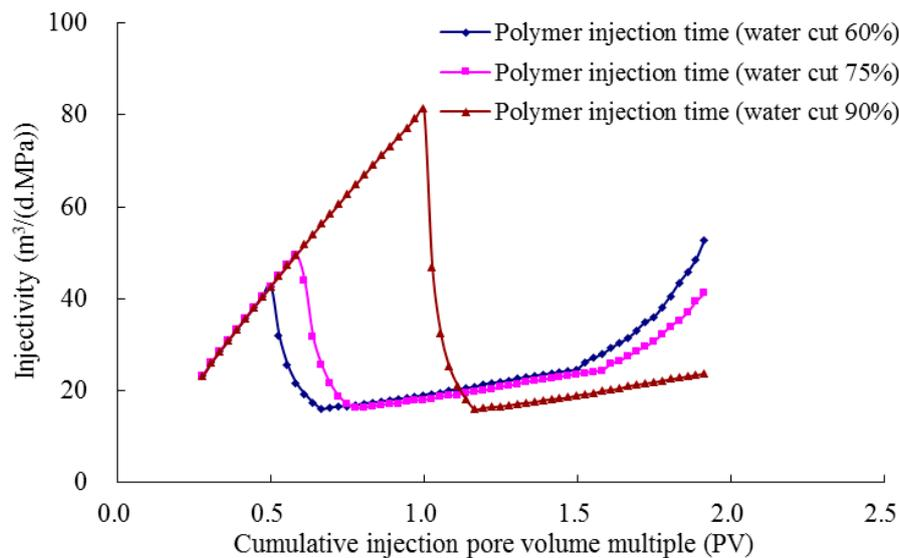
Figure 10. The influence of polymer injection time on injectivity.
