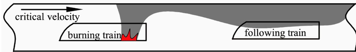
Figure 1. Schematic diagram of longitudinal ventilation.
