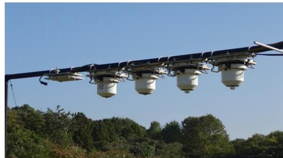
**Figure 2.** Photos of (a) BSRN instruments (GHI, DNI, and DIF, Source from the web site of JMA aerological observatory [http://www.jma-net.go.jp/kousou/obs\\_third\\_div/rad/rad\\_sol.html](http://www.jma-net.go.jp/kousou/obs_third_div/rad/rad_sol.html)) and (b) measurements of upward longwave radiation (ULW) instruments at Japan Meteorological Agency's (JMA) aerological observatory.
