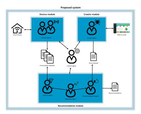
Figure 1. Architecture of the proposed multiagent system.
