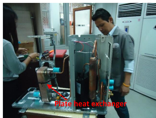
Figure 7. Modification of the air-source heat pump (ASHP) and installation of the plate heat exchanger.
