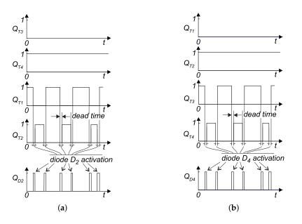
**Figure 7.** Gate signals when: (**a**) positive half-period output voltage is required; and (**b**) negative half-period output voltage is required.
