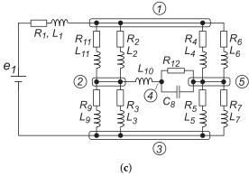
Figure 3. (a) Oriented graph; (b) Tie-set matrix graph; and (c) Circuit elements.
