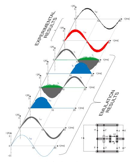
Figure 13. Results of emulation and measurement currents.
