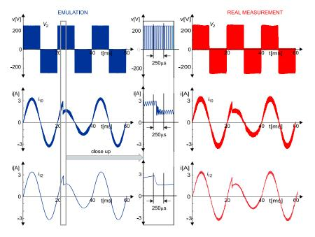
Figure 12. Emulation results and its close-up (blue curves) and measured results (red curves).
