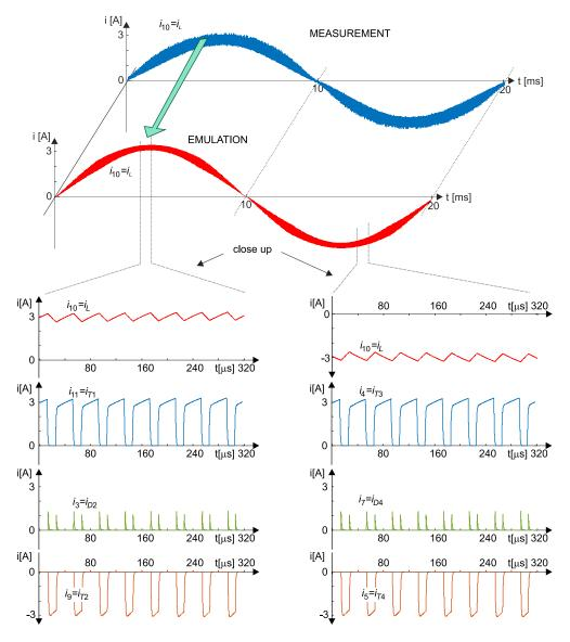
**Figure 14.** Emulation and measurement results of inductor current and close up of emulated: inductor current ( $i_{10}$ ), MOSFETs currents ( $i_4$ ,  $i_5$ ,  $i_9$  and  $i_{11}$ ) and diodes currents ( $i_3$  and  $i_7$ ).
