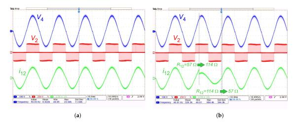
**Figure 11.** Load measurements (x-axis 10 ms/div): (**a**) constant load resistance, voltages; blue curve  $V_4$ , y-axis 100 V/div; red curve  $V_2$ , y-axis 250 V/div; current, green curve  $i_{12}$ , y-axis 2.5 A/div; and (**b**) step change into load resistance, voltages; blue curve  $V_4$ , y-axis 100 V/div; red curve  $V_2$ , y-axis 250 V/div; current, green curve  $i_{12}$ , y-axis 2.5 A/div.
