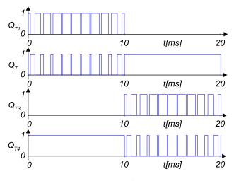
**Figure 5.** Gate signals:  $Q_{T1}$ – $Q_{T4}$ .
