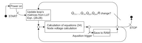
Figure 10. System emulator state diagram.
