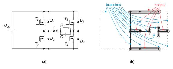
Figure 2. (a) Electrical circuit DC-AC converter; and (b) circuit graph.
