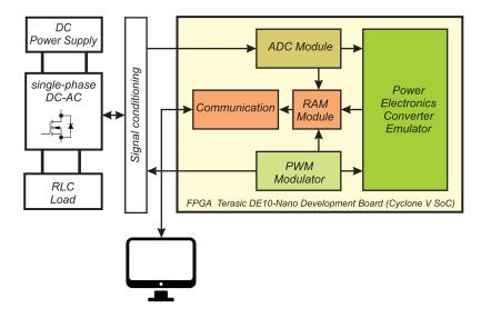
Figure 1. The emulator and real DC-AC system architecture appropriate for testing and verification.
