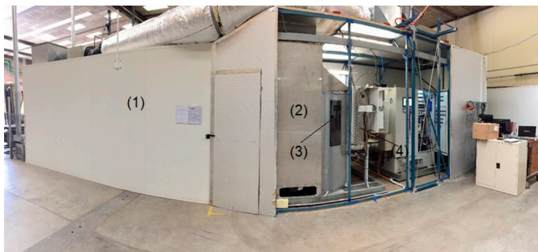
Figure 5. UniSA Test Chamber: (1) Prechamber, (2) Main Chamber, (3) DPC, (4) Gas Cooler (photo credit: BHI-UniSA).
