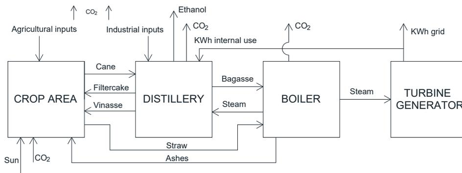
Figure 1. General flowchart of the process (mass and energy).
