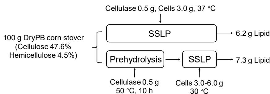
**Figure 4.** The mass balance of microbial lipid production from DryPB corn stover using SSLP process and PreSSLP process.
