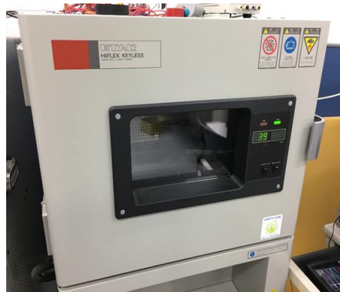
Figure A1. Thermo-hygrostat (HIFLEX KEYFLESS TL401E).
