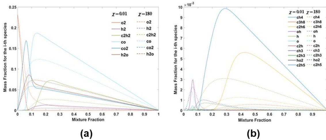
**Figure 1.** Flamelet profiles applied in the combustion model for: (a) Major chemical species; (b) Minor and intermediate chemical species for scalar dissipation rates of 0.01 (near chemical equilibrium) and 180 (approaching flame extinction).
