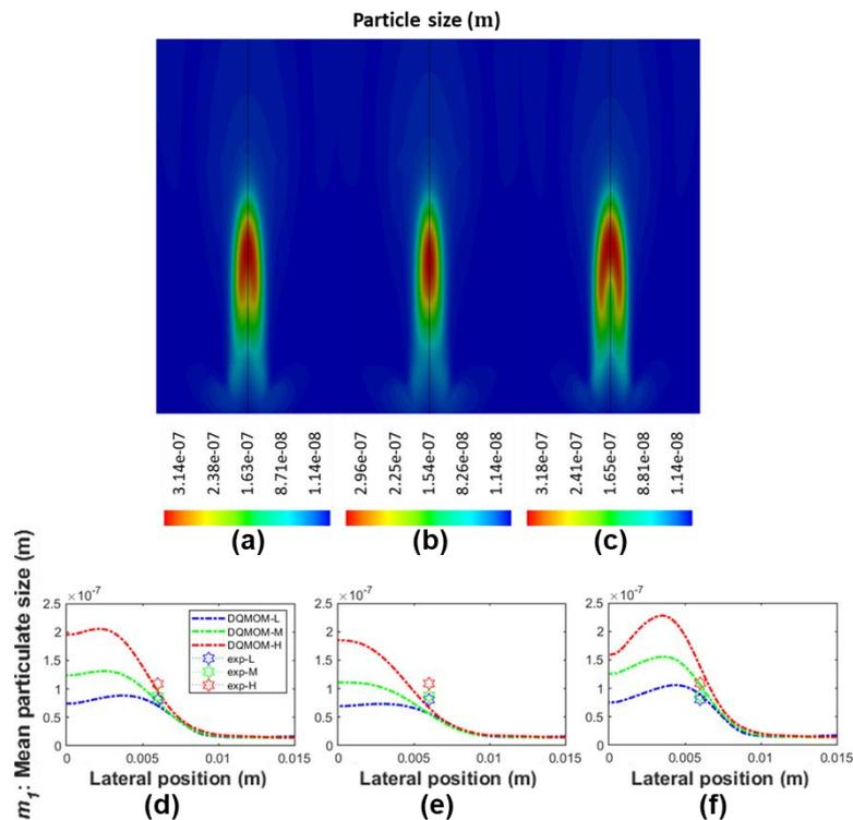
**Figure 18.** Contour plot of soot particle size, evaluated from: Schmidt number of (a) 0.7, (b) 0.5, and (c) 0.9, and X-Y plot of soot particle size at selected HABs, evaluated from: Schmidt number of (d) 0.7, (e) 0.5, and (f) 0.9 as compared with experimental result.
