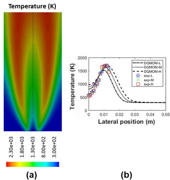
**Figure 2.** (a) Temperature contour plot and (b) comparisons of numerical and experimental temperature distributions at three vertical height levels above the burner.
