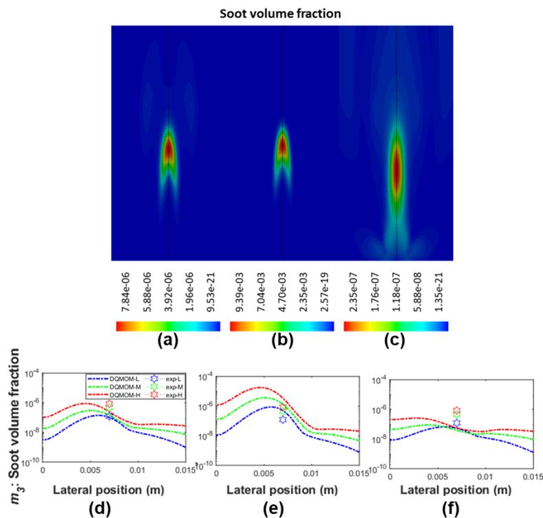
**Figure 15.** Contour plot of soot volume fraction, evaluated from: fractal dimension of (a) 2.0, (b) 1.8, and (c) 2.2, and X-Y plot of soot volume fraction at selected HABs, evaluated from: fractal dimension of (d) 2.0, (e) 1.8, and (f) 2.2 as compared with experimental result.
