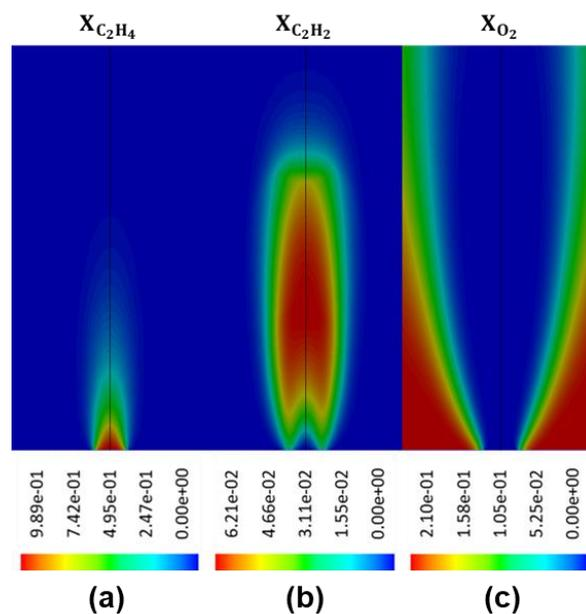
**Figure 3.** Contour plot of the mole fraction of reacting species: (a) ethylene,  $X_{C_2H_4}$ ; (b) acetylene,  $X_{C_2H_2}$ ; and, (c) oxygen,  $X_{O_2}$ .
