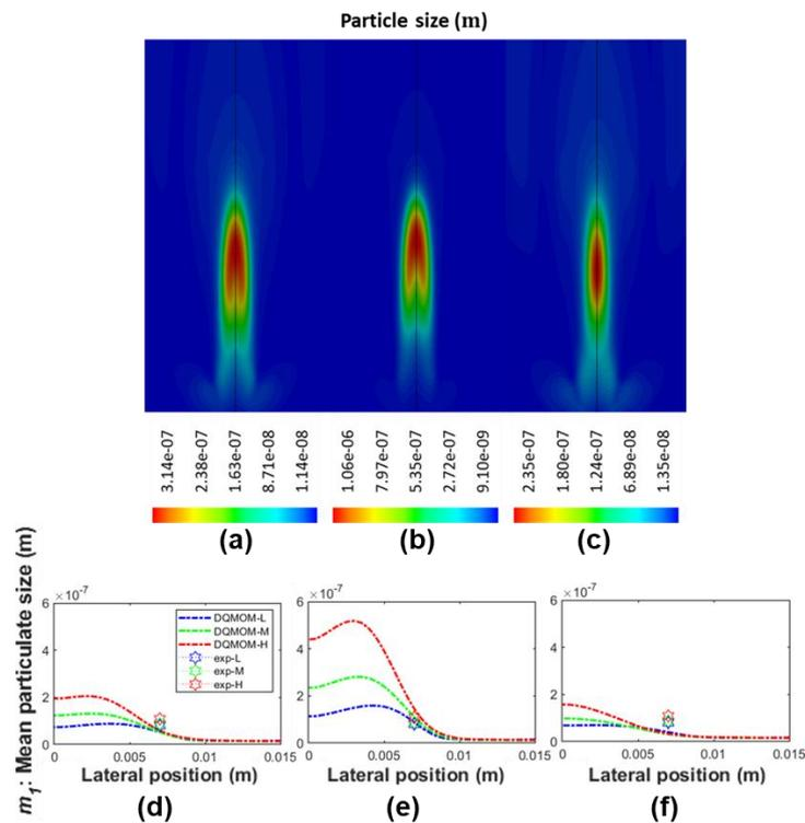
**Figure 14.** Contour plot of soot particle size, evaluated from: fractal dimension of (a) 2.0, (b) 1.8, and (c) 2.2, and X-Y plot of soot particle size at selected HABs, evaluated from: fractal dimension of (d) 2.0, (e) 1.8, and (f) 2.2 as compared with experimental result.
