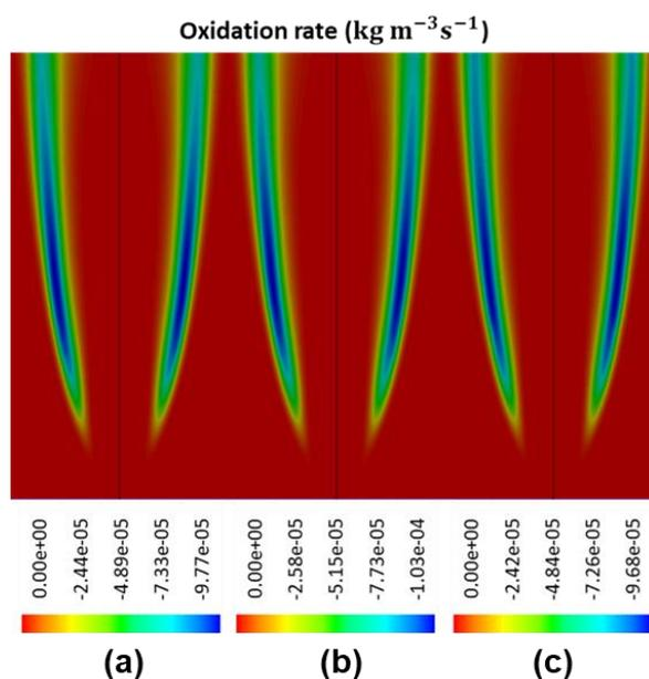
**Figure 12.** Contour plot of oxidation rate, evaluated from: fractal dimension of (a) 2.0, (b) 1.8, and (c) 2.2.
