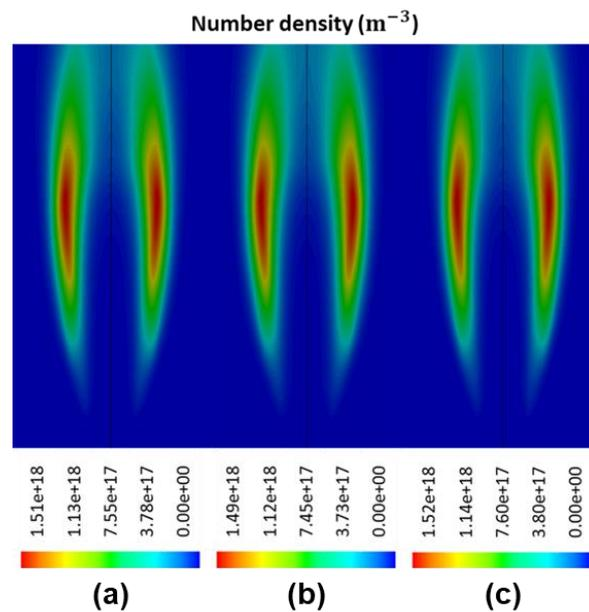
**Figure 16.** Contour plot of soot number density, evaluated from: Schmidt number of (a) 0.7, (b) 0.5, and (c) 0.9.
