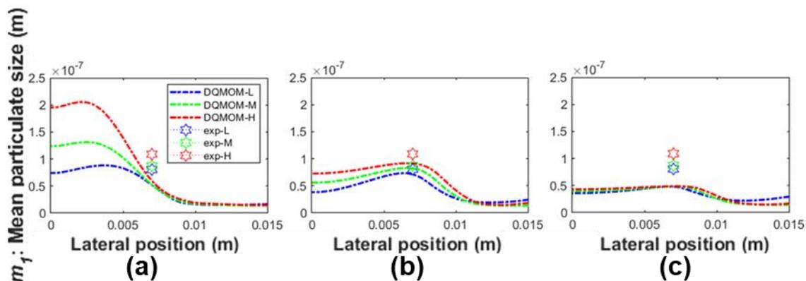
**Figure 6.** X-Y plot of soot particle size at selected height above burners (HABs), evaluated from: (a) Moss law; (b) Leung law; and, (c) Fairweather law as compared with experimental result.
