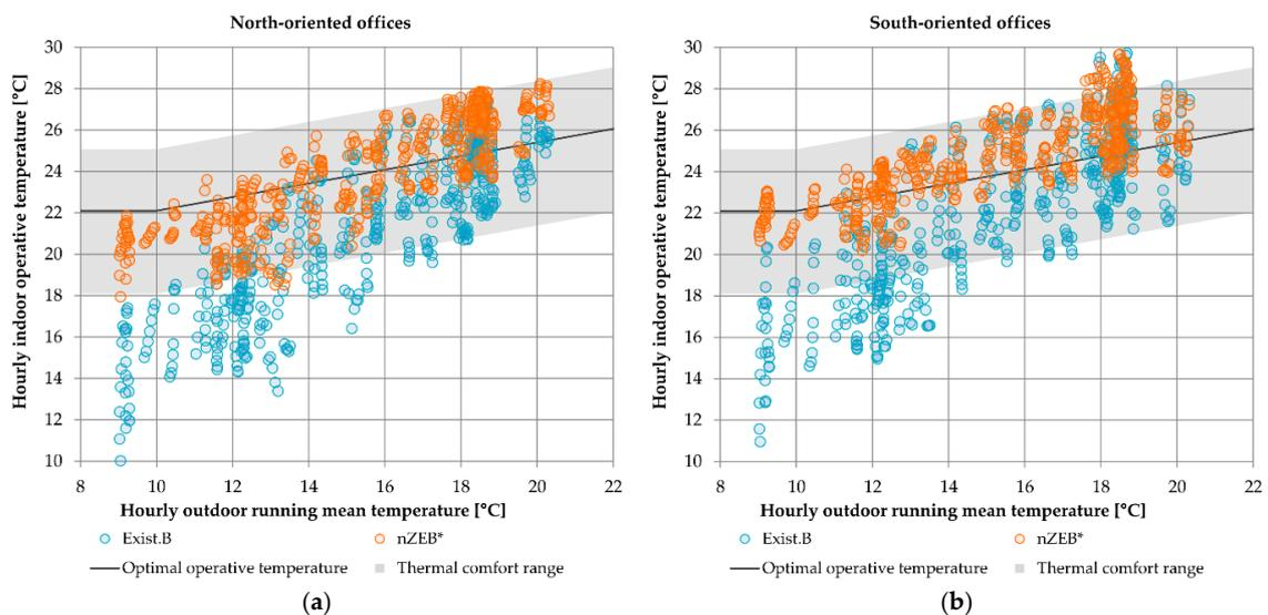
**Figure 5.** Thermal comfort analysis results; comparison between the building storey in the current condition (Exist.B) and considering the retrofitting of the building envelope (nZEB\*): (a) North-oriented offices; (b) South-oriented offices.
