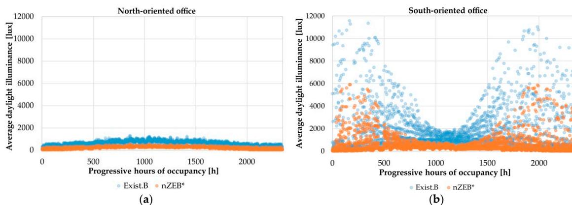
**Figure 6.** Comparison of the average hourly values of daylight illuminance for the occupied hours over the whole year between the building in the present configuration (Exist.B) and after retrofitting of the building envelope (nZEB\*): (a) North-oriented offices; (b) South-oriented offices.
