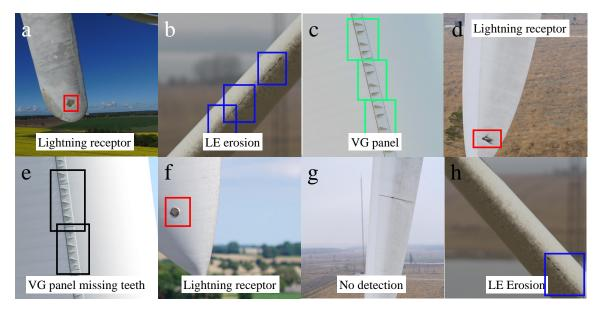
**Figure 6.** Suggestion results on the test images for the trained model using Inception-ResNet-V2 together with the proposed augmentation schemes.
