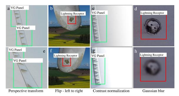
Figure 3. Illustrations of the regular augmentation methods applied to drone inspection images.
