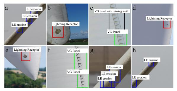
Figure 2. Examples of manually-annotated damages related to wind turbine blades. LE, Leading Edge.
