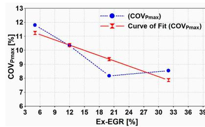
**Figure 9.** Cyclic variability of  $P_{max}$  due to variation of Ex-EGR setting (rpm = 3000, IMEP = 2.1 bar,  $T_{epc} = 425\text{--}530$  K).
