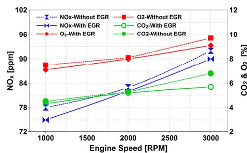
**Figure 15.** Influence of In/Ex-EGR on  $\text{NO}_x$ ,  $\text{CO}_2$  and  $\text{O}_2$  concentrations at idling and low/mid-load settings (rpm = 1000–3000, IMEP = 1–2.1 bar,  $T_{epc}$  = 385–530 K, AFR = 14–16).
