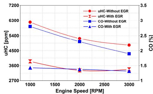
**Figure 14.** Influence of In/Ex-EGR on uHC and CO concentrations at idling and low/mid-load settings (rpm = 1000–3000, IMEP = 1–2.1 bar,  $T_{epc}$  = 385–530 K, AFR = 14–16).
