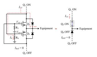
Figure 7. Mutual blocking when the main power supply is restored.
