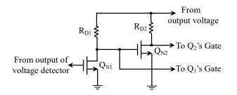
Figure 3. A control logic circuit consisting of two NMOS transistors.
