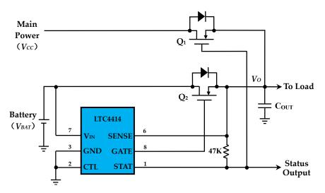
Figure 5. Typical application circuit of LTC4414. Source: Linear Technology Corporation.
