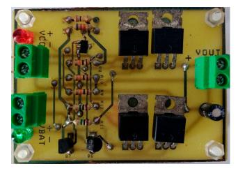
Figure 10. Circuit implementation of the proposed dual power source switch.
