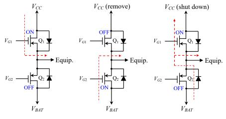
(a) Only main power or both (b) Only battery (c) Main power shut down
