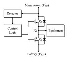
Figure 2. Switching control architecture using main power detection.
