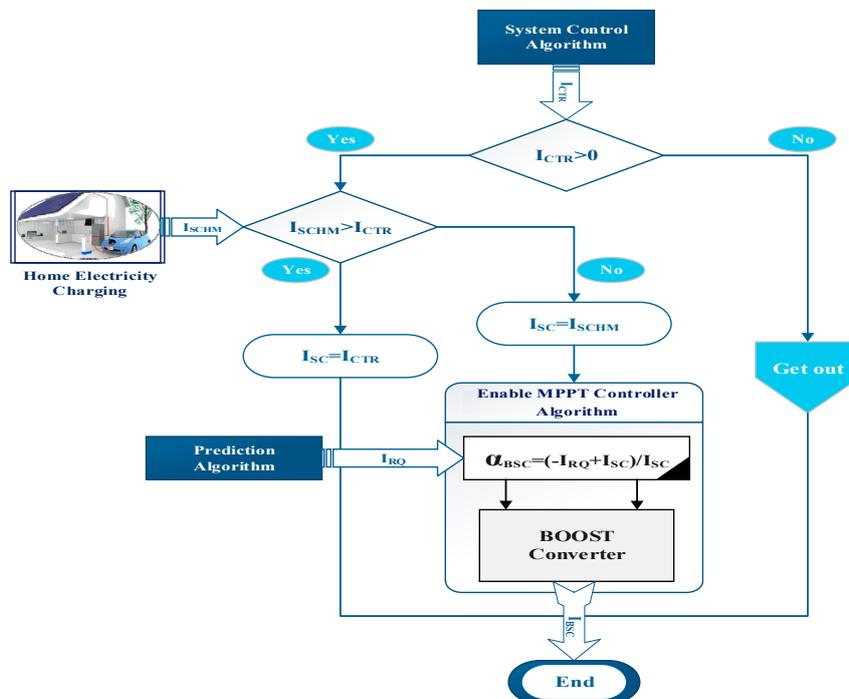
Figure 4. Emergency control algorithm.
