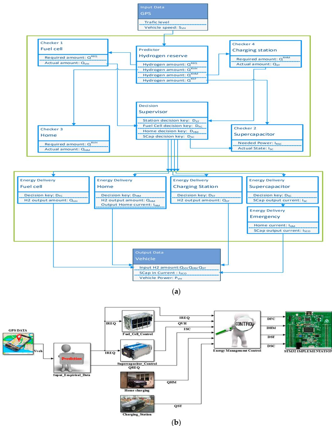
Figure 6. NZE-HEVSim tool simulation: (a) Simulation diagram and (b) MATLAB/Simulink model.
