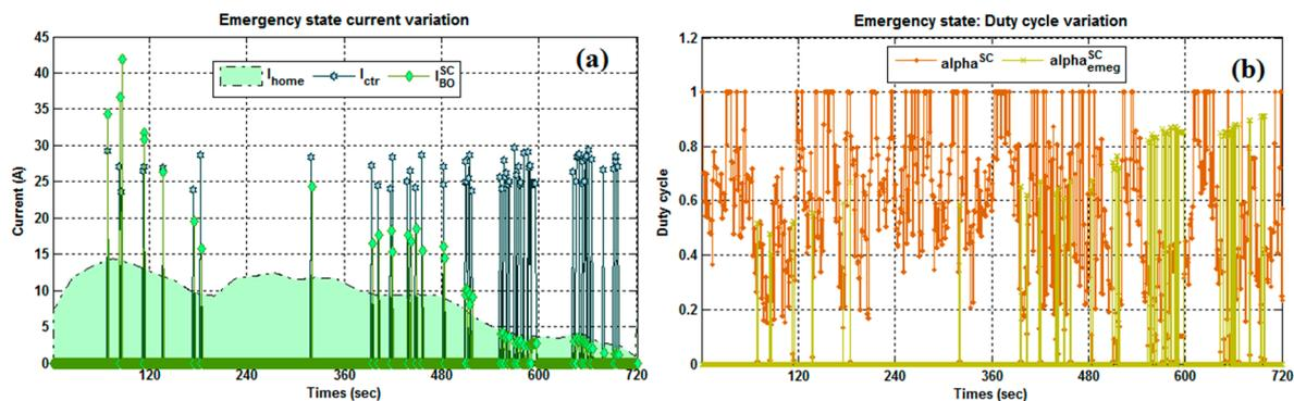
Figure 12. Emergency state: (a) SCap current variation and (b) duty cycle variation.
