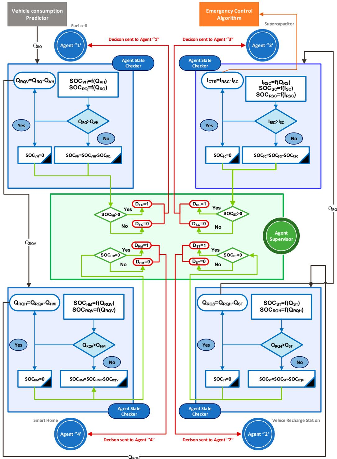
Figure 5. Agent communication control algorithm.
