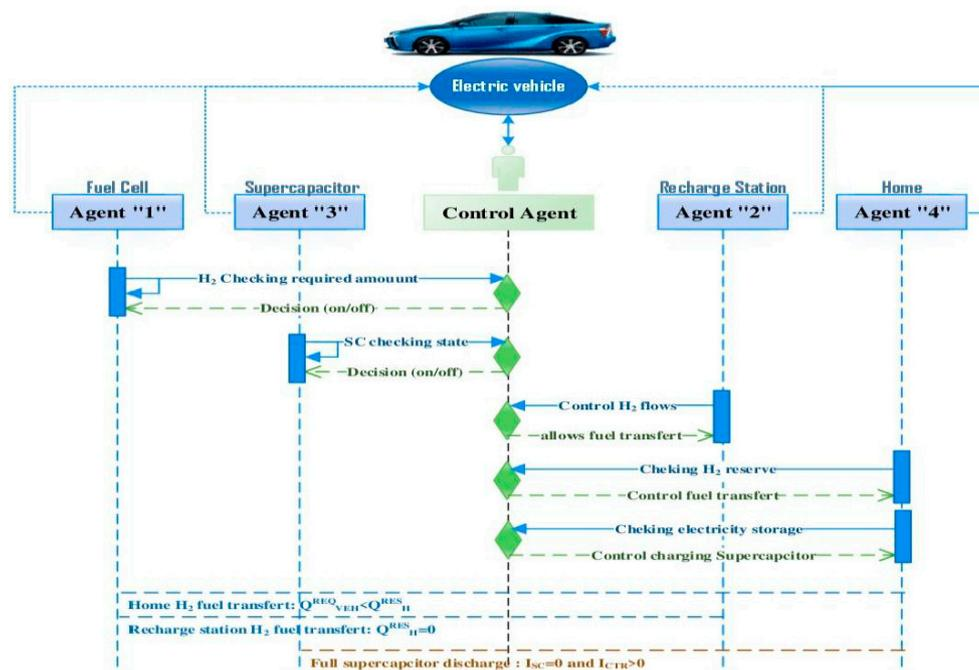
Figure 2. Sequence diagram for distribution flow control.
