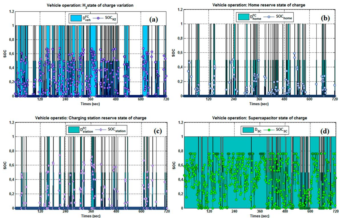
**Figure 10.** SOC variation and decision key per component: (a) FC; (b) home; (c) charging station; and (d) supercapacitor.
