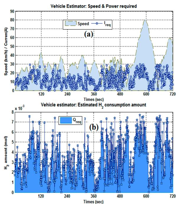
Figure 8. Vehicle estimator outputs: (a) speed estimation and (b) required H<sub>2</sub> amount.
