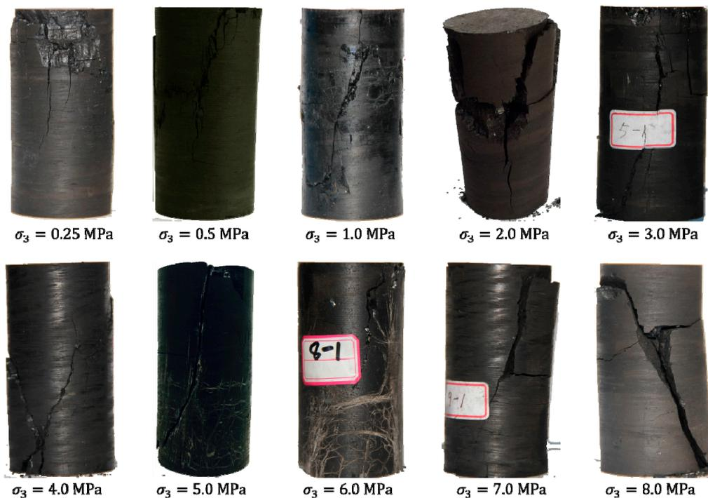
**Figure 8.** Failure pattern evolution with the increase of confining stress.
