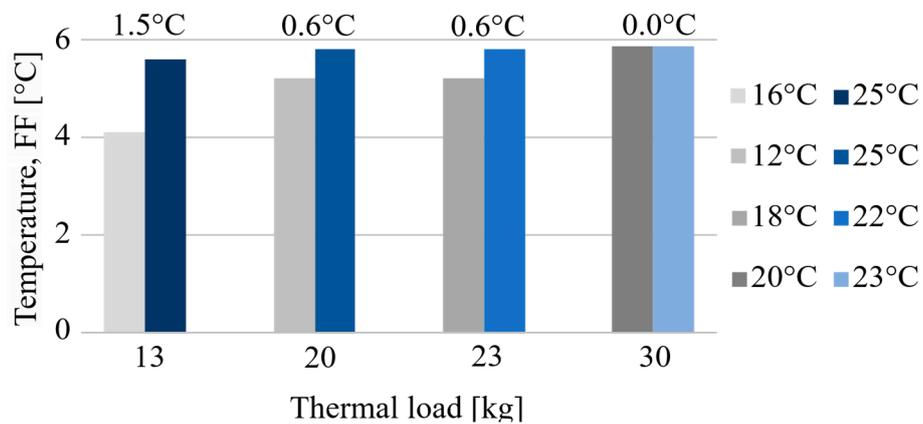
**Figure 7.** Temperature in the fresh-food compartment maintaining the constant thermal load at two ambient temperature conditions.
