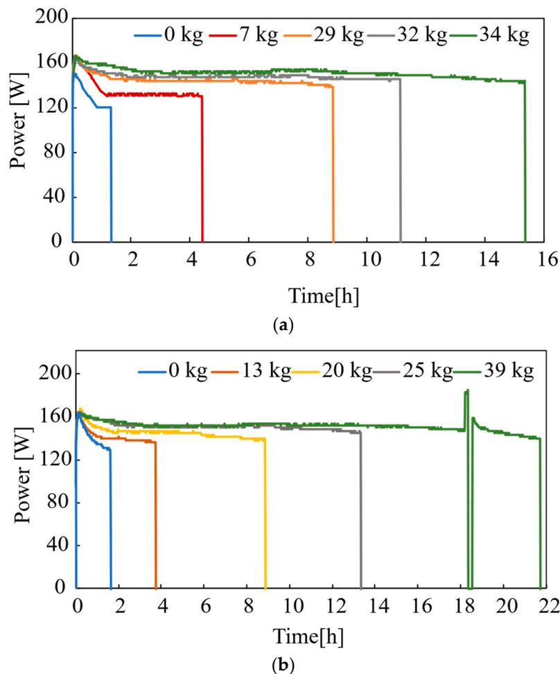
**Figure 6.** Power during the first on-state of the compressor: (a) room temperature at 20 °C; (b) room temperature at 25 °C.
