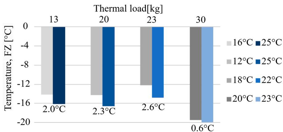
**Figure 8.** Temperature in the freezer compartment maintaining a constant thermal load at two temperature conditions.
