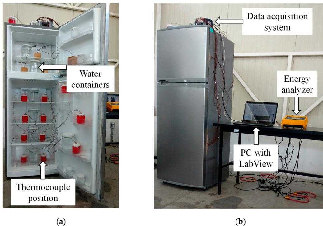
**Figure 2.** Experimental test bench: (a) temperature distribution; (b) instrumentation.
