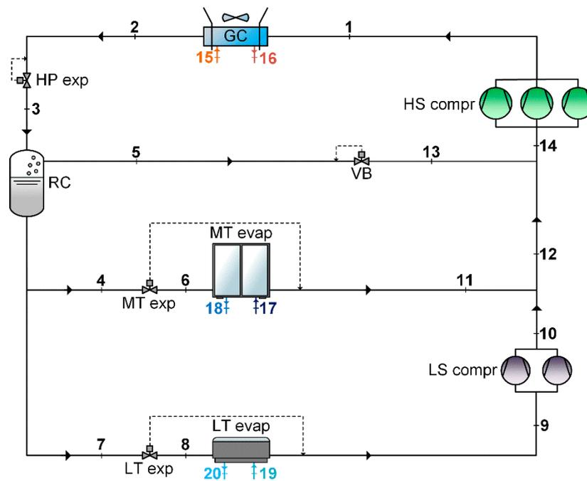
**Figure 1.** Schematic of a conventional transcritical R744 booster supermarket refrigeration system (CB) (GC: air-cooled R744 gas cooler/condenser; HP exp: high pressure expansion valve; HS compr: high stage compressor rack; VB: vapor by-pass valve; RC: receiver; MT exp: expansion valve (medium temperature); MT evap: evaporates at medium temperature; LT exp: expansion valve (low temperature); LT evap: evaporates at low temperature; LS compr: low stage compressor rack).
