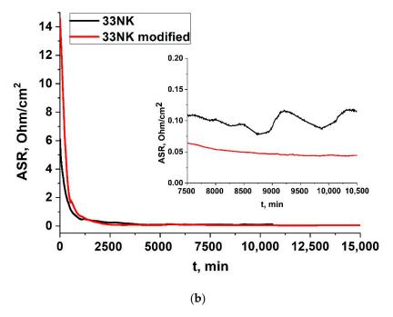
**Figure 13.** Dependences of the electrical resistance of the 33NK alloy samples without and with surface modification on temperature (**a**) and time at  $T = 850 \,^{\circ}\text{C}$  (**b**).
