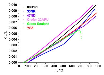
**Figure 3.** Dependences of the relative change in the linear size of the samples of the 33NK and 47ND alloys, the 08H17T and Crofer 22APU steels, glass sealant, and  $Zr_{0.8}Y_{0.2}O_{3-\delta}$  (YSZ) electrolyte on temperature.
