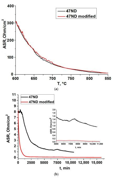
**Figure 14.** Dependences of the electrical resistance of the 47ND alloy samples without and with surface modification on temperature (**a**) and time at T = 850 °C (**b**).
