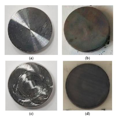
**Figure 2.** The 33NK (a) and 47ND (c) alloys samples before the modification procedure, and the 33NK (b) and 47ND (d) alloys samples after the modification procedure and the annealing in a high-vacuum installation.
