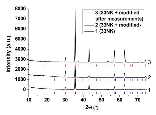
**Figure 8.** Grazing incidence XRD patterns of the 33NK alloy without surface modification (1), with modification (2), and with modification after the electrical conductivity measurement test (3). Colored vertical lines indicate the position of the angles of the allowed Bragg reflections: Red ones confirm the presence of the isostructural spinel-like phases, such as  $Fe_3O_4$ ,  $CoFe_2O_4$ ,  $NiFe_2O_4$ ,  $NiMn_2O_4$ , etc. Blue confirms the presence of  $Fe_2O_3$ .
