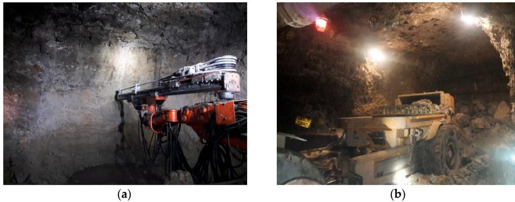
**Figure 5.** Forehead of exploitation room: (a) Drilling blasting holes; (b) Discharge point of output.
