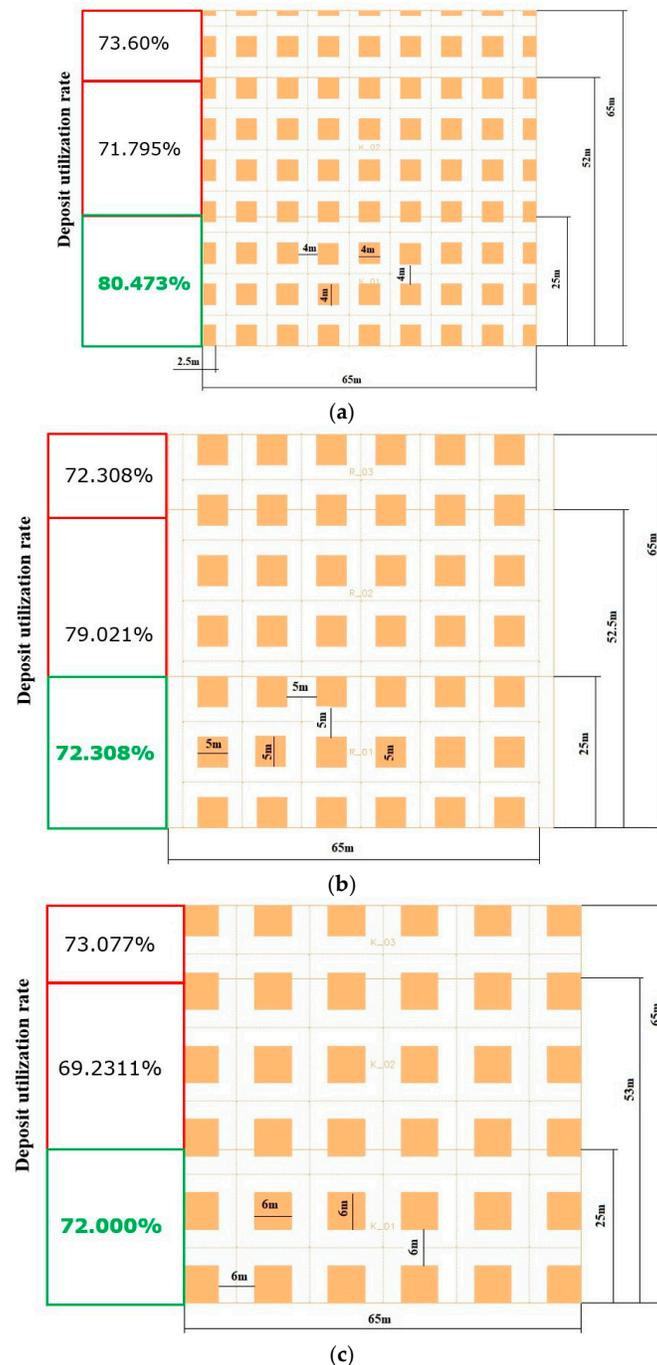
Figure 4. Room and pillar method with variable geometry: (a) 4 m × 4 m; (b) 5 m × 5 m; (c) 6 m × 6 m.
