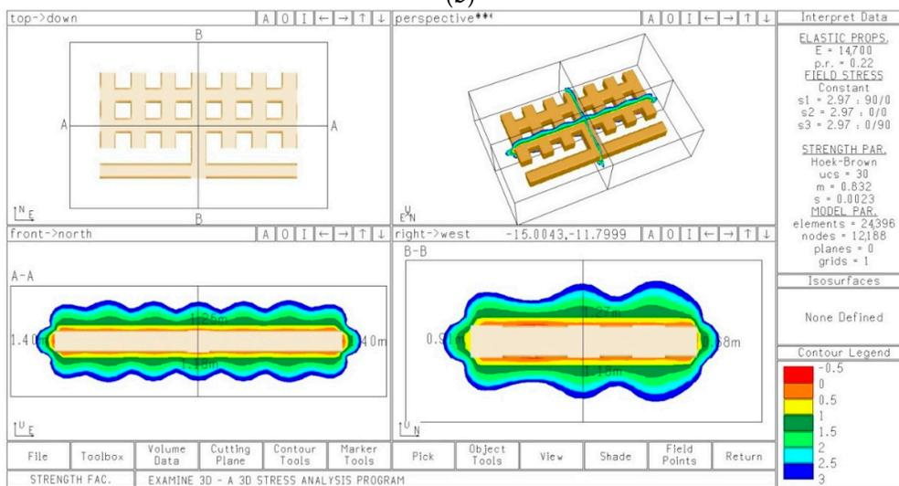
**Figure 7.** Ranges of the rock destruction zone around excavations for the geometry of the room and pillar method: (a) 4 m × 4 m; (b) 5 m × 5 m; (c) 6 m × 6 m.
