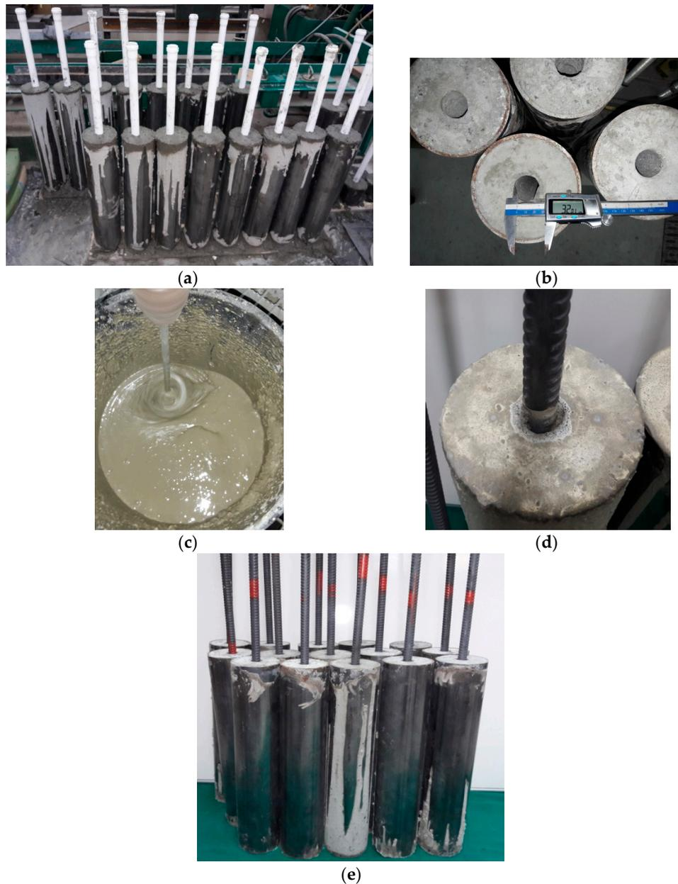
**Figure 10.** Preparation for tests: (a) View of steel cylinders with polyester pipes with an outer diameter of 32 mm; (b) Diameter of the hole in the concrete block; (c) Mixing of the binder; (d) Bolt rod embedded on the cement binder; (e) View of installed bolt rods to steel cylinders filled with concrete.
