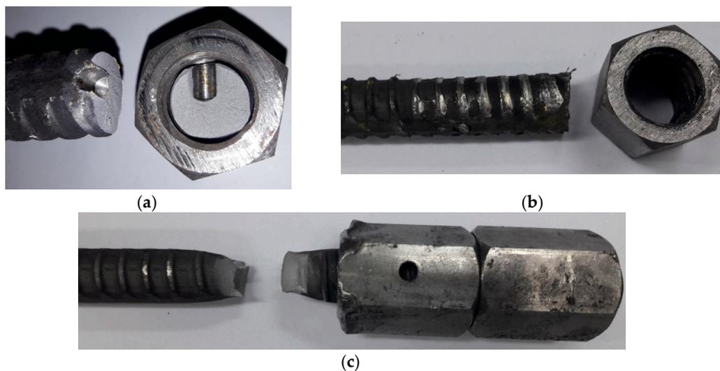
**Figure 15.** Loss of support load capacity through: (a) Break on the rod in place of the spiro pin; (b) Thread cutting; (c) Break on the bolt rod.
