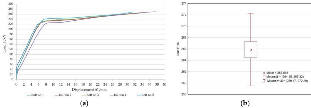
Figure 12. Load-displacement characteristic of the SAS 650/800 rock bolt support with a flat washer and one nut: (a) Characterization course; (b) Load range.
