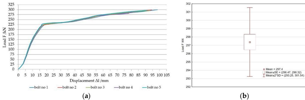
**Figure 13.** Load-displacement characteristic of the SAS 650/800 rock bolt support with a shaped washer and one nut: (a) Characterization course; (b) Load range.
