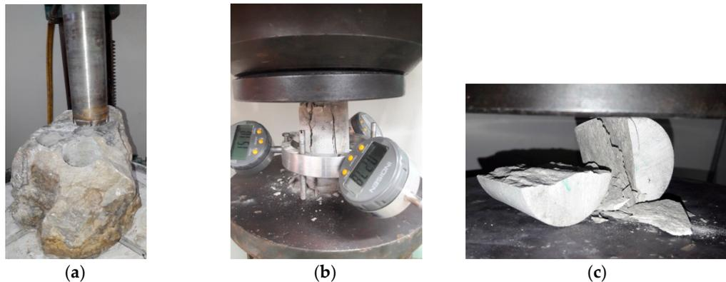
**Figure 6.** Dolomite samples: (a) Cutting out regular samples; (b) Sample after the compression test; (c) Sample after the tensile test.
