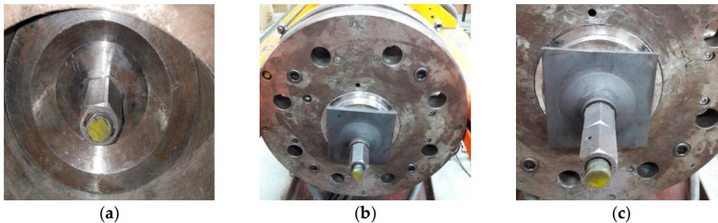
**Figure 9.** Configuration of the bolt rod and nut connection: (a) Flat washer; (b) Shaped washer and one nut; (c) Shaped washer and two nuts.
