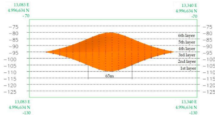
Figure 3. Division of the deposit into 5 m thick layers (-80 to -110).
