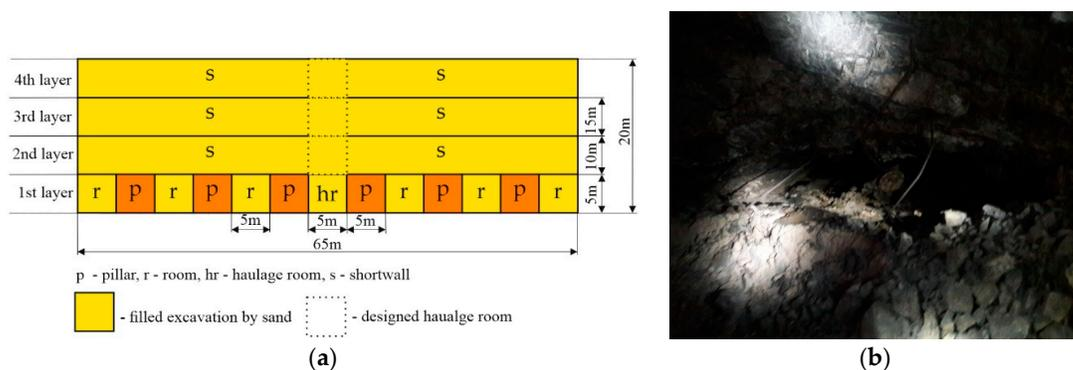
**Figure 1.** Exploitation of a thick ore deposit: (a) Division into layers; (b) View of rock bolts and fillings from the first layer.
