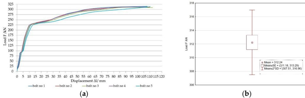
**Figure 14.** Load-displacement characteristic of the SAS 650/800 rock bolt support with a shaped washer and two nuts: (a) Characterization course; (b) Load range.
