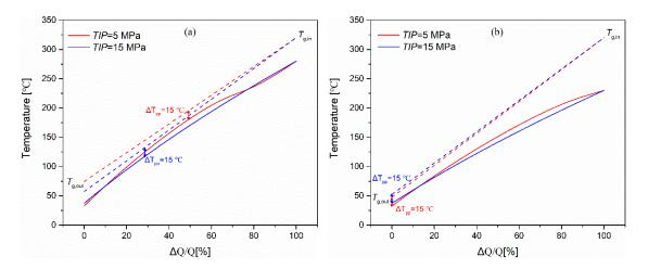
**Figure 12.** Temperature matching between the heat source and working fluid for the OTC: (**a**) Turbine inlet temperature =  $280 \degree C$ ; (**b**) Turbine inlet temperature =  $230 \degree C$ .
