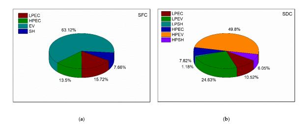
Figure 20. Distribution of the exergy loss in HRSG. (a) SFC; (b) SDC.
