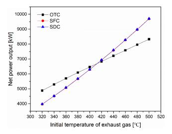
**Figure 21.** The maximum net power output of OTC, SFC, and SDC under the various initial temperature of exhaust gas.
