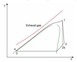
Figure 2. T-s diagram of the organic trans-critical cycle.
