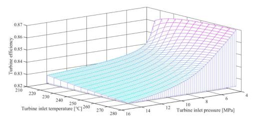
Figure 10. Effects of the turbine inlet pressure and temperature on the turbine efficiency.
