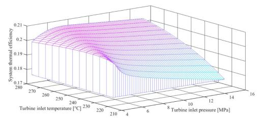
Figure 9. Effects of the turbine inlet pressure and temperature on the system thermal efficiency.
