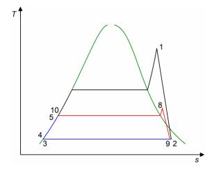
Figure 7. T-s diagram of the steam dual-pressure cycle.
