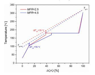
Figure 15. Thermal matching between the heat source and working fluid for the SFC.
