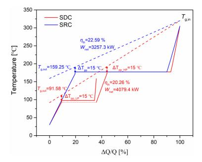
Figure 17. T-Q diagram of the heat source and working fluid for the SDC and basic SRC.
