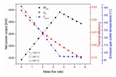
Figure 14. Effect of mass flow ratio on the system performance of SFC.
