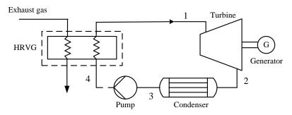
Figure 1. Schematic diagram of the organic trans-critical cycle.
