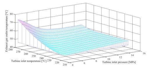
Figure 11. Effects of the turbine inlet pressure and temperature on the exhaust gas outlet temperature.
