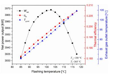
Figure 16. Effect of flashing temperature on the system performance of SFC.
