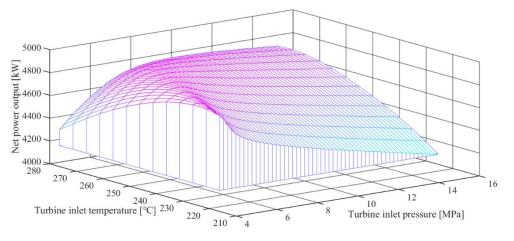
Figure 13. Effects of turbine inlet pressure and temperature on the system net power output.
