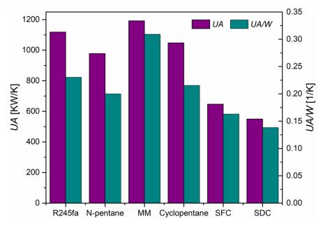
Figure 19. The UA and UA/W of HRSG for the OTC, SFC, and SDC.
