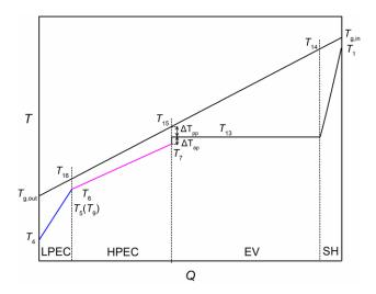
Figure 5. T-Q diagram of flue gas and working fluid in the HRSG of steam flash cycle.
