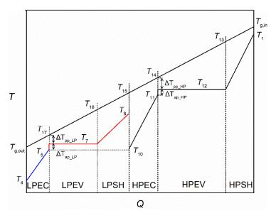
Figure 8. T-Q diagram of flue gas and working fluid in the HRSG of SDC.
