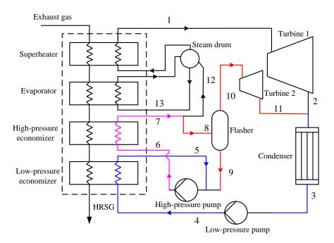
Figure 3. Schematic diagram of the steam flash cycle.
