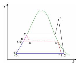
Figure 4. T-s diagram of the steam flash cycle.
