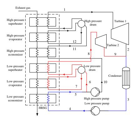
Figure 6. Schematic diagram of the steam dual-pressure cycle.
