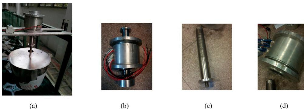
**Figure 12.** Tubular PM linear generator with single translators for comparison: (a) experimental platform of D-DWECs; (b) prototype; (c) translator; (d) stator and windings.
