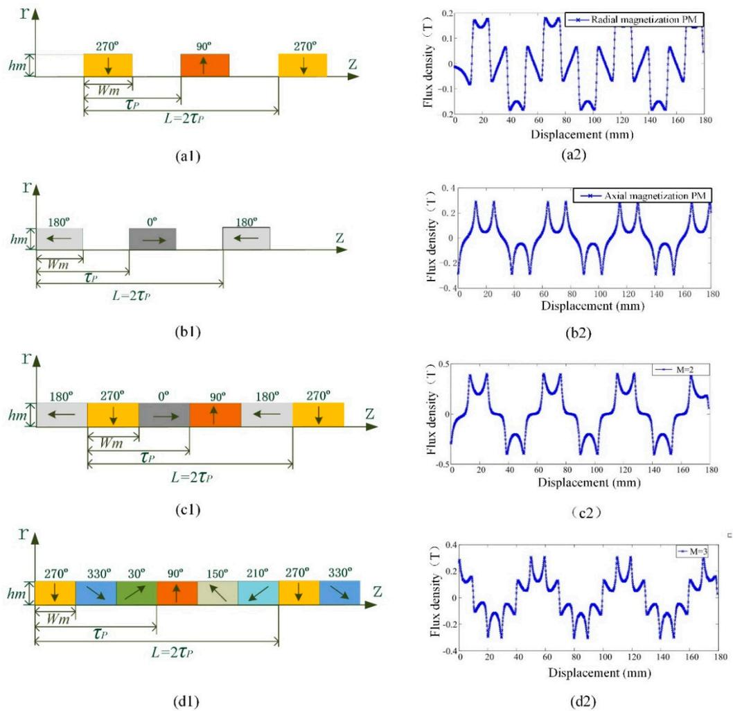
**Figure 3.** PM arrays structure model and flux density curve: (a1) radial magnetization PM structure, (b1) axial magnetization PM structure, (c1)  $n = 2$  Halbach PM structure, (d1)  $n = 3$  Halbach PM structure, (a2), (b2), (c2) and (d2) are the gap flux densities of Figures 3a1, 3b1, 3c1 and 3d1, respectively.
