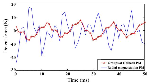
**Figure 10.** Detent force of TPMLG with groups of Halbach PM magnetized structure and radial magnetization PM.
