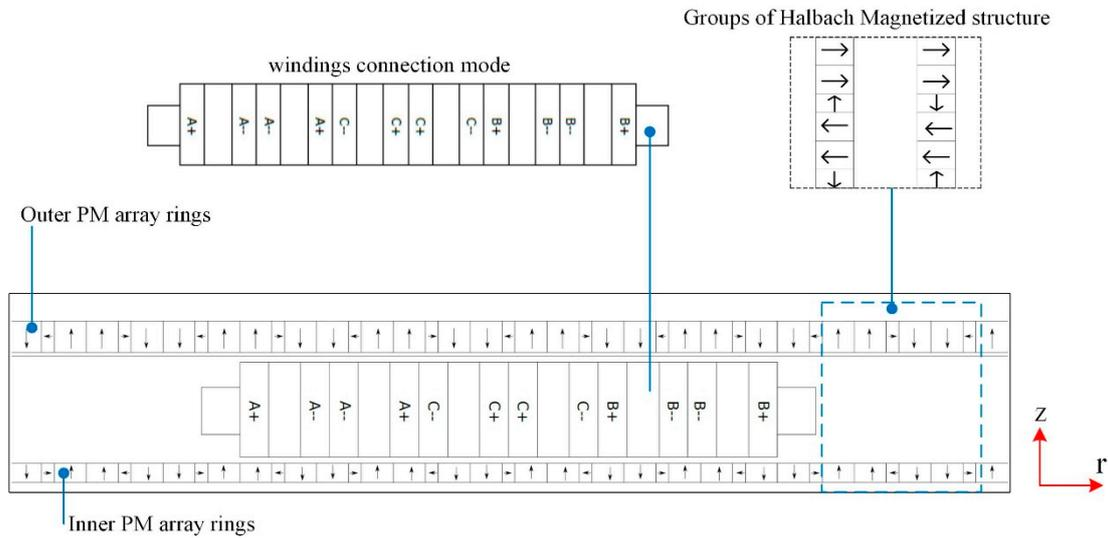
**Figure 5.** Two-dimensional (2D) mode with groups of Halbach PM magnetized structure and windings connection.
