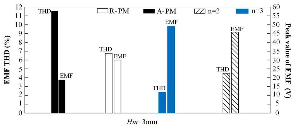
**Figure 4.** THD and EMF of the linear generator with the four PM structure.
