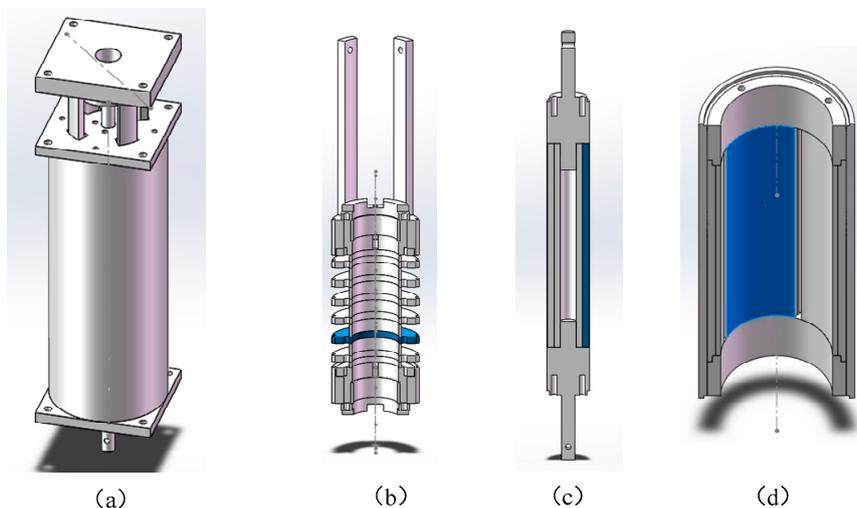
**Figure 13.** Proposed tubular linear PM generator (TPMLG) with double translators for D-DWECs: (a) three-dimensional (3D) schematic; (b) stator; (c) inner translator; (d) outer translator.
