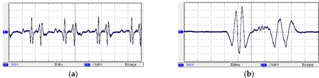
**Figure 15.** Output voltage waveform of experimental platform of D-DWECs. (a) Wave height is 0.15 m, wave period is 1.5 s. (b) Wave height is 0.2 m, wave period is 2 s.
