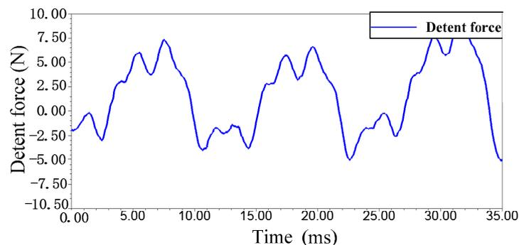
**Figure 9.** Detent force of the TPMLG with double translators.
