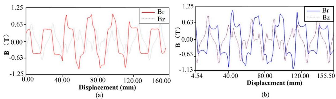
**Figure 8.** Air gap flux density curves of generator: (a) air gap flux density of inner translator and (b) air gap flux density of outer translator.
