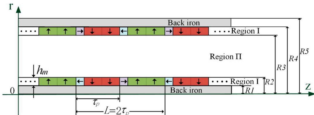
**Figure 6.** Analysis region with groups of Halbach PM magnetized structure.
