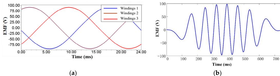
**Figure 11.** Electromotive force (EMF) waveforms of the TPMLG: (a) at constant velocity (b) at sine velocity.
