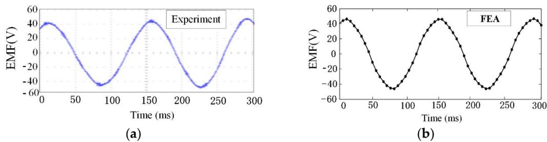
**Figure 14.** EMF waveform of the generator with single translator: (a) in the experiment, (b) with the finite element method (FEM).
