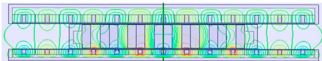
Figure 7. Magnet field distribution of generator.
