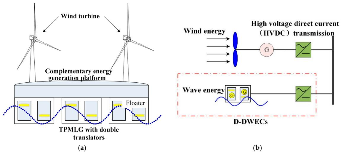
**Figure 1.** The complementary energy generation platform: (a) the configuration of platform; (b) the configuration of power take-off (PTO).
