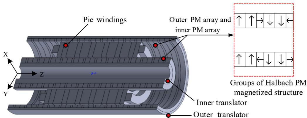
**Figure 2.** Structure of TPMLG with double translators.
