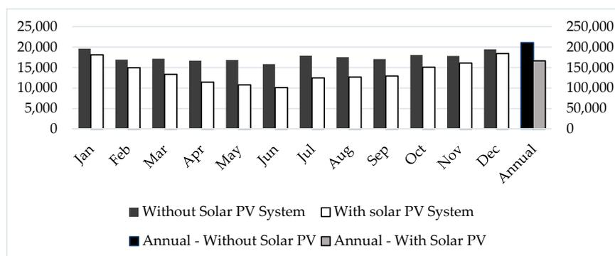
Figure 6. Annual electricity demand on grid of the project without and with solar PV system.
