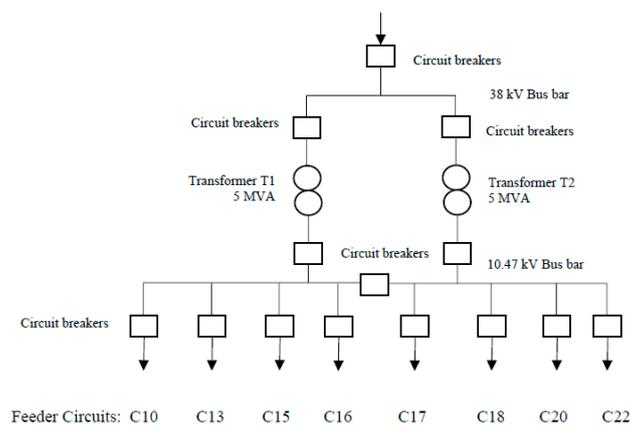
Figure 1. Primary substation single line diagram [32].
