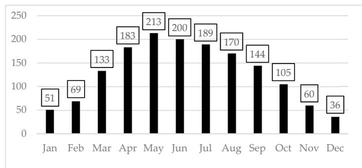
Figure 5. Annual solar PV electricity generation (kWh) of a single residential unit.
