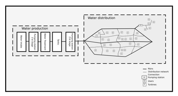
**Figure 1.** The scheme of the water supply system.
