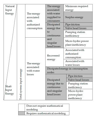
Figure A2. Energy balance for water supply system [30].
