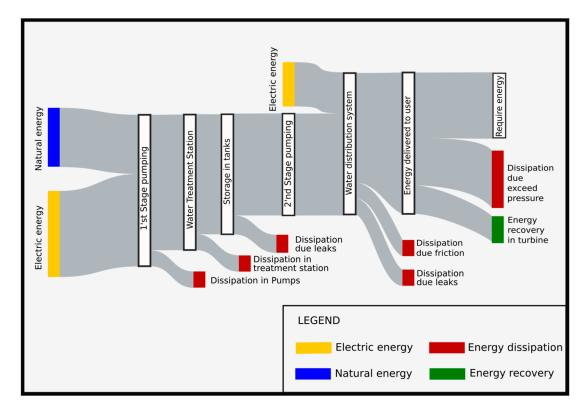
Figure 2. Scheme of energy transformation in a water supply system.
