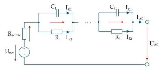
Figure 3. Equivalent circuit models (ECM) of the battery cell.
