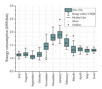
Figure 11. Boxplot analysis of energy consumption (kWh/km).
