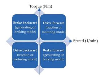
Figure 5. Motor speed-torque diagram (traction modes).
