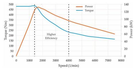
Figure 6. Motor speed-torque/power characteristic.
