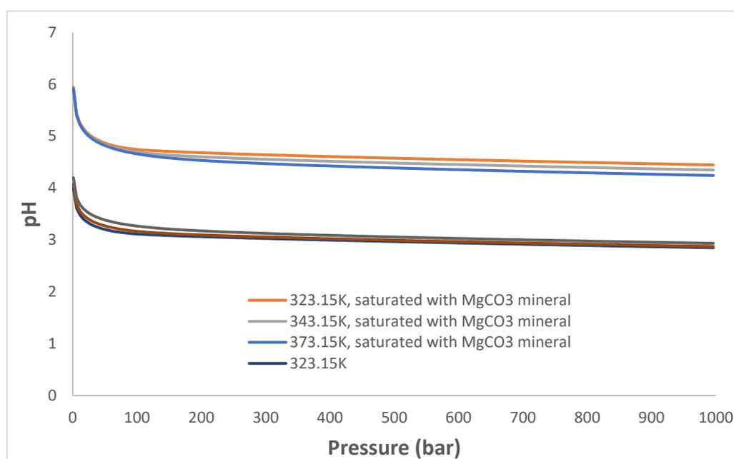
**Figure 7.** pH of solutions at various temperatures and pressures with or without  $\text{MgCO}_3$  saturated.
