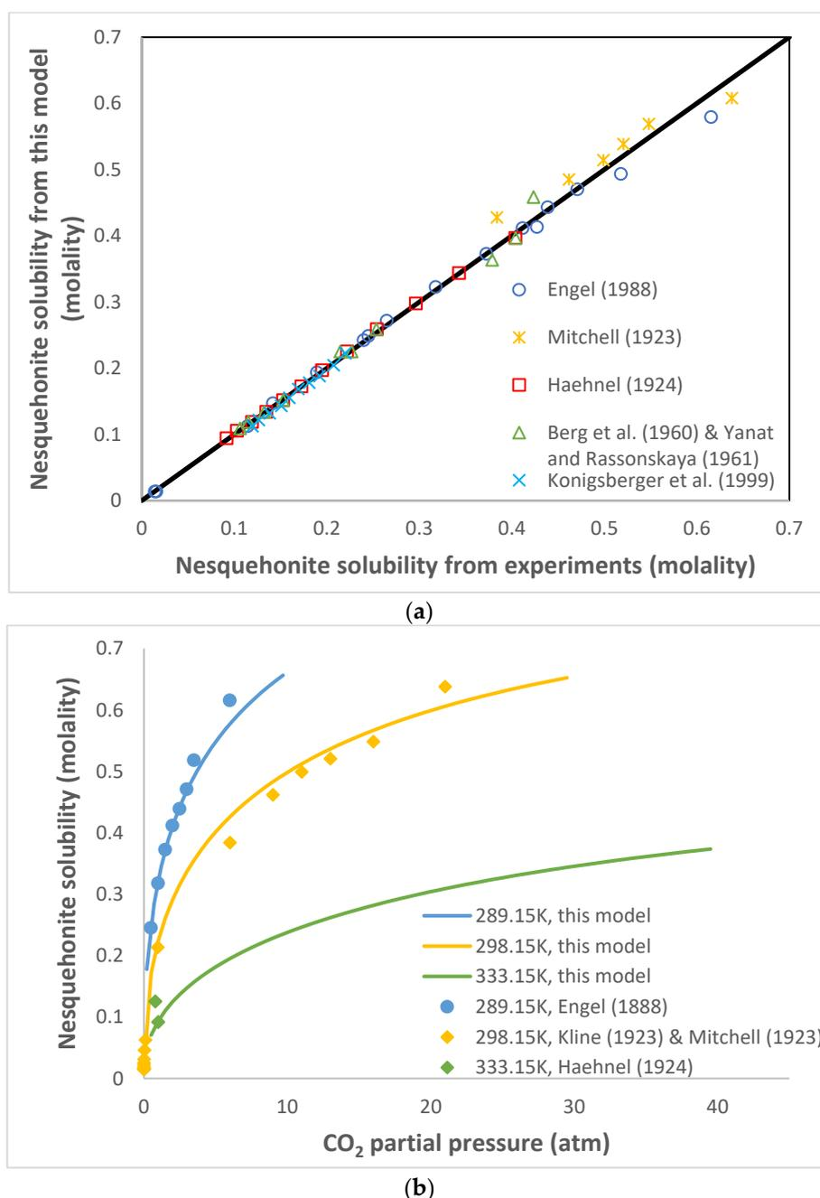
**Figure 2.** Comparison of nesquehonite solubility in water at various temperatures and pressures between calculated results by this model and experiments. Dots are experimental data from references [10,13–17], and lines are calculated results by this model. (a) comparison of experimental nesquehonite solubility in water and the calculated results by this model. (b) Nesquehonite solubility varying with CO<sub>2</sub> partial pressure at various temperatures.
