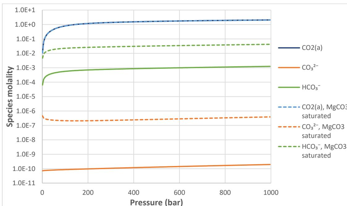
**Figure 8.** Carbonate concentrations varying with pressure under conditions of  $\text{MgCO}_3$  saturated or  $\text{MgCO}_3$  free. The solid lines represent the results with  $\text{MgCO}_3$  free and dashed lines represent the results with  $\text{MgCO}_3$  saturated.
