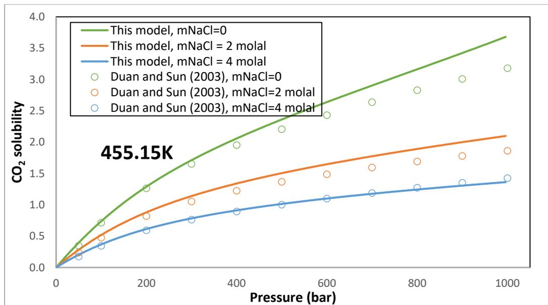
**Figure 4.** CO<sub>2</sub> solubility varying with pressure at different NaCl concentration calculated by this model (lines) and DS model (dots).
