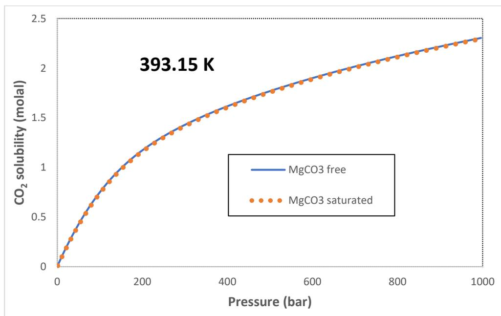
**Figure 5.** CO<sub>2</sub> solubility varying with pressure at 393.15 K in solutions with MgCO<sub>3</sub> saturated (dots) or free (line) conditions.
