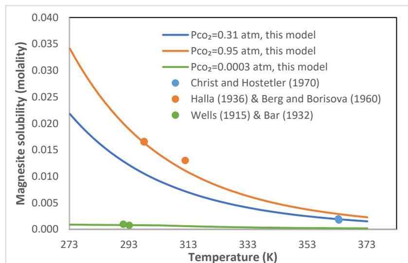
**Figure 1.** Comparison of magnesite solubility in water at various temperatures and pressures. Lines are calculated results by this model, and dots are from experiments.
