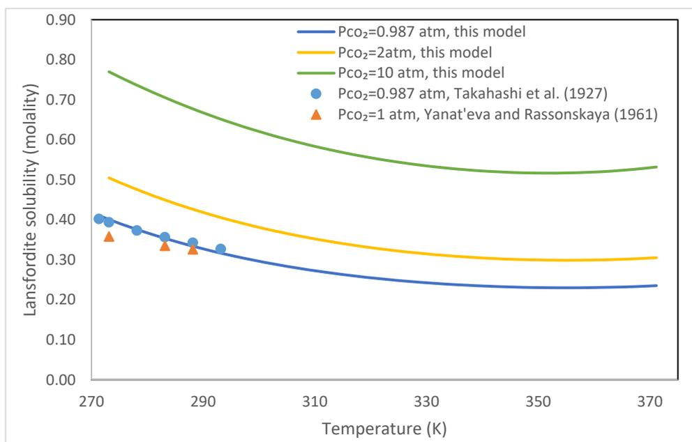
**Figure 3.** Comparison of lansfordite solubility in water at various temperatures and pressures. Line is the calculated results by this model and dots are from experiments.
