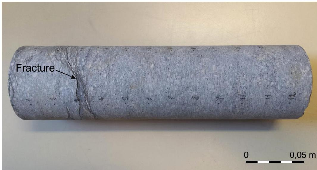
**Figure 17.** Image of a core sample of Macroforaminifera limestone showing fractures developed during the water saturation process.
