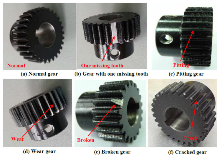
Figure 4. Six types of planetary gear states.
