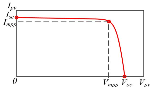
Figure 7. Characteristic of photovoltaic cells.
