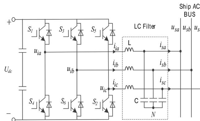
Figure 8. Circuit of the investigated inverter.
