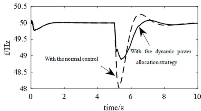
Figure 19. Frequency response curves of the micro-grid system.
