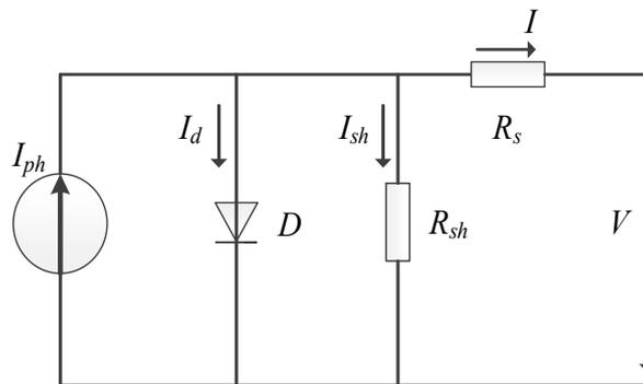
Figure 6. Equivalent circuit of photovoltaic cells.
