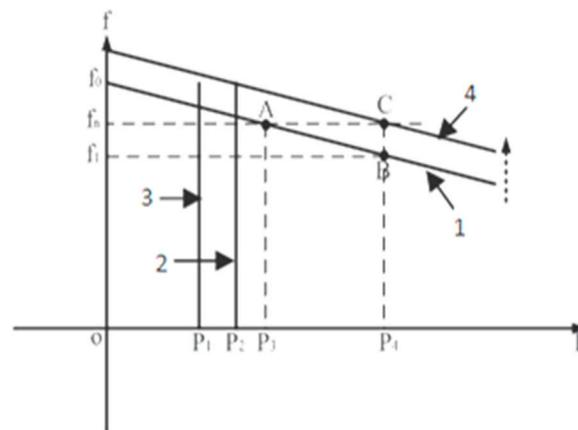
Figure 11. Frequency static regulation process.
