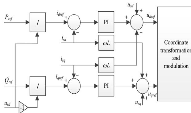
Figure 9. Power control (PQ) control strategy of inverter.
