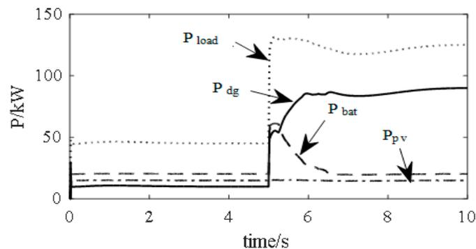
Figure 20. Operational profiles of different energy modules.
