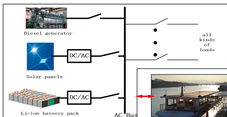
**Figure 5.** Proposed structure of ship's micro-grid system.
