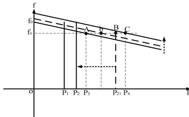
Figure 13. The proposed static frequency regulation process.
