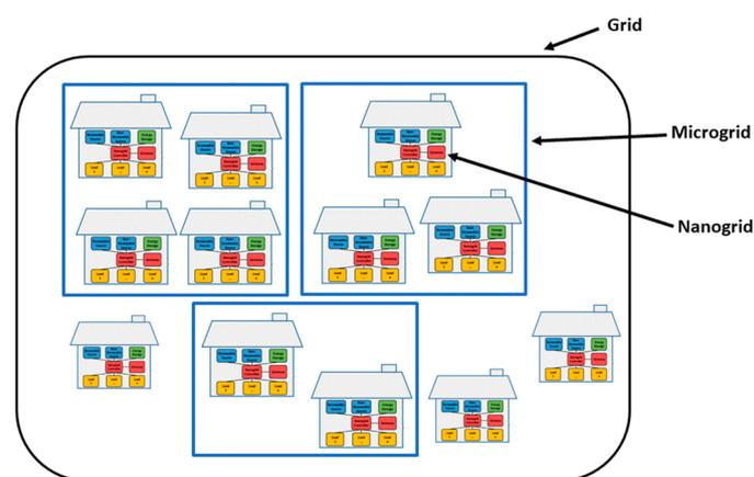
**Figure 3.** An overall comparison between micro-grid and nano-grid.
