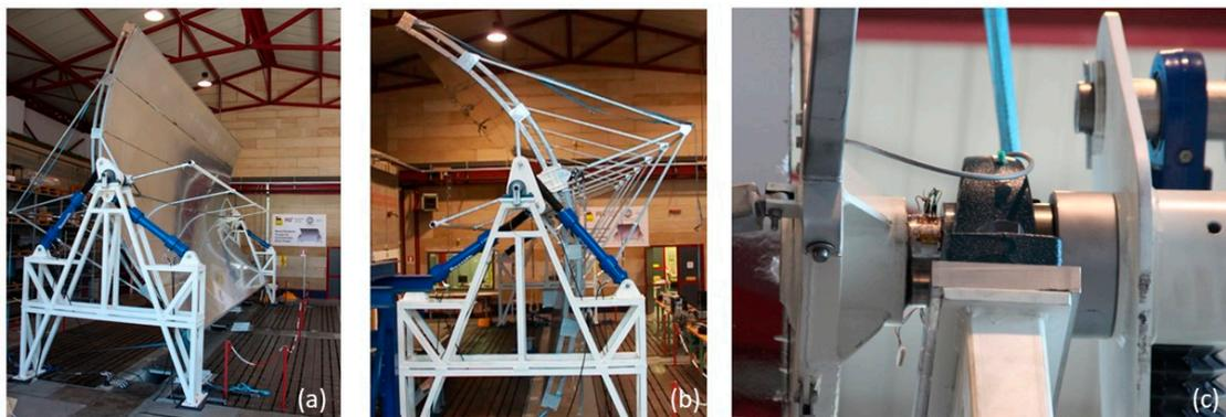
Figure 2. (a) Overview of the parabolic trough collector prototype; (b) Side view of the trough rotated at  $-110^\circ$  and its support structure; (c) Detail of the shaft and the torsional strain gauges.
