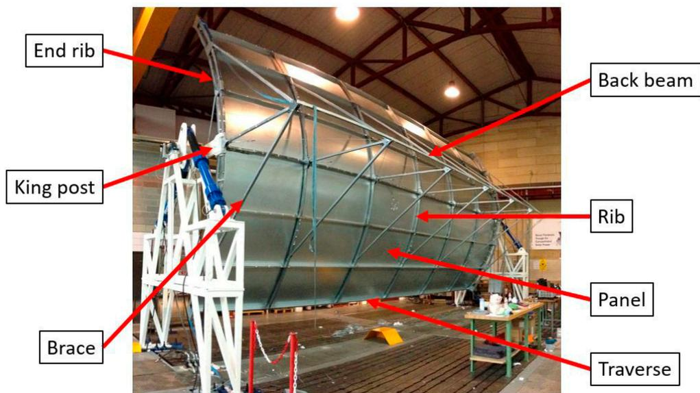
Figure 1. Main components of the parabolic trough collector.
