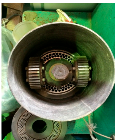
Figure 2. Flat die pellet machine.
