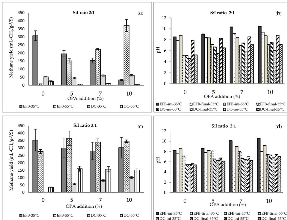
**Figure 1.** Methane production yield and pH from (SS-AD) of empty fruit bunches (EFB) and decanter cake (DC) at S:I ratio 2:1 and 3:1 with various % Oil palm ash (OPA) addition. Methane yield (a) and pH (b) at S:I ratio 2:1; Methane yield (c) and pH (d) at S:I ratio 3:1.
