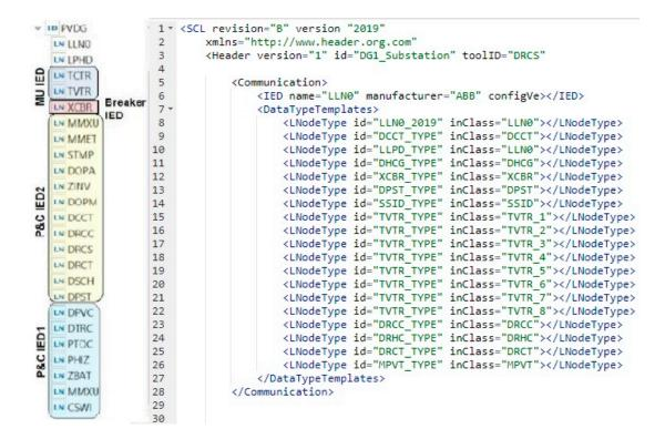
Figure 4. SCD file example for PV IED packed information.
