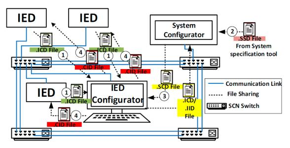
Figure 2. SCL file configuration for typical SCN.
