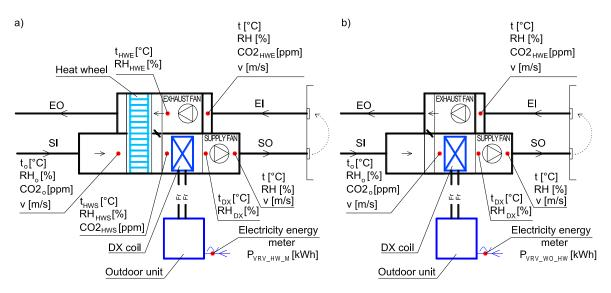
**Figure 3.** Schematic diagram (**a**) for the placement of the measurement points on the real operating AHU and (**b**) the AHU without a heat recovery operation assumption.
