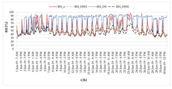
Figure 6. The air relative humidity values in the air handling processes.
