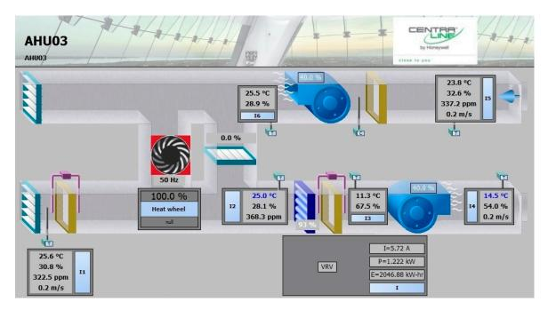
Figure 4. A screenshot of the investigated AHU in the Building Management System (BMS).
