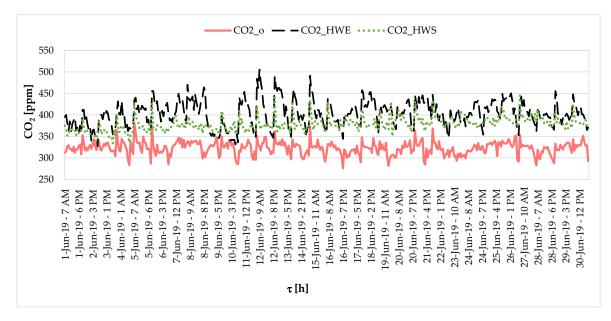
Figure 11. The carbon dioxide values in the investigated supply and exhaust sections of the heat wheel.
