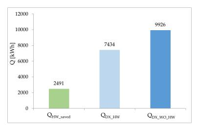
Figure 9. The energy recovery and auxiliary cooling energy consumption for ventilation.
