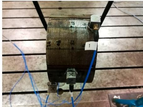
Figure 8. Stator core modal experiment.
