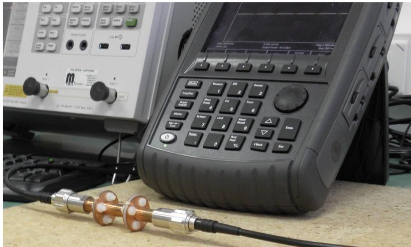
Figure 15. Measurement setup for characterization of adiabatic line-scattering parameters.
